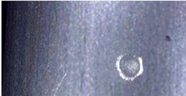
Figure 20.16.3-1: MMOD Impact Damage
