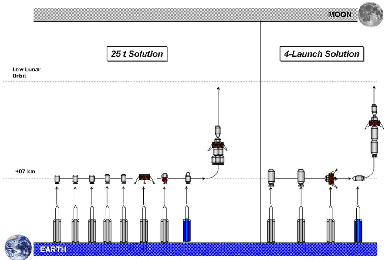
**Figure 7.4-3: Earth Orbit Departure Configuration for 25 t Launch Solution**
