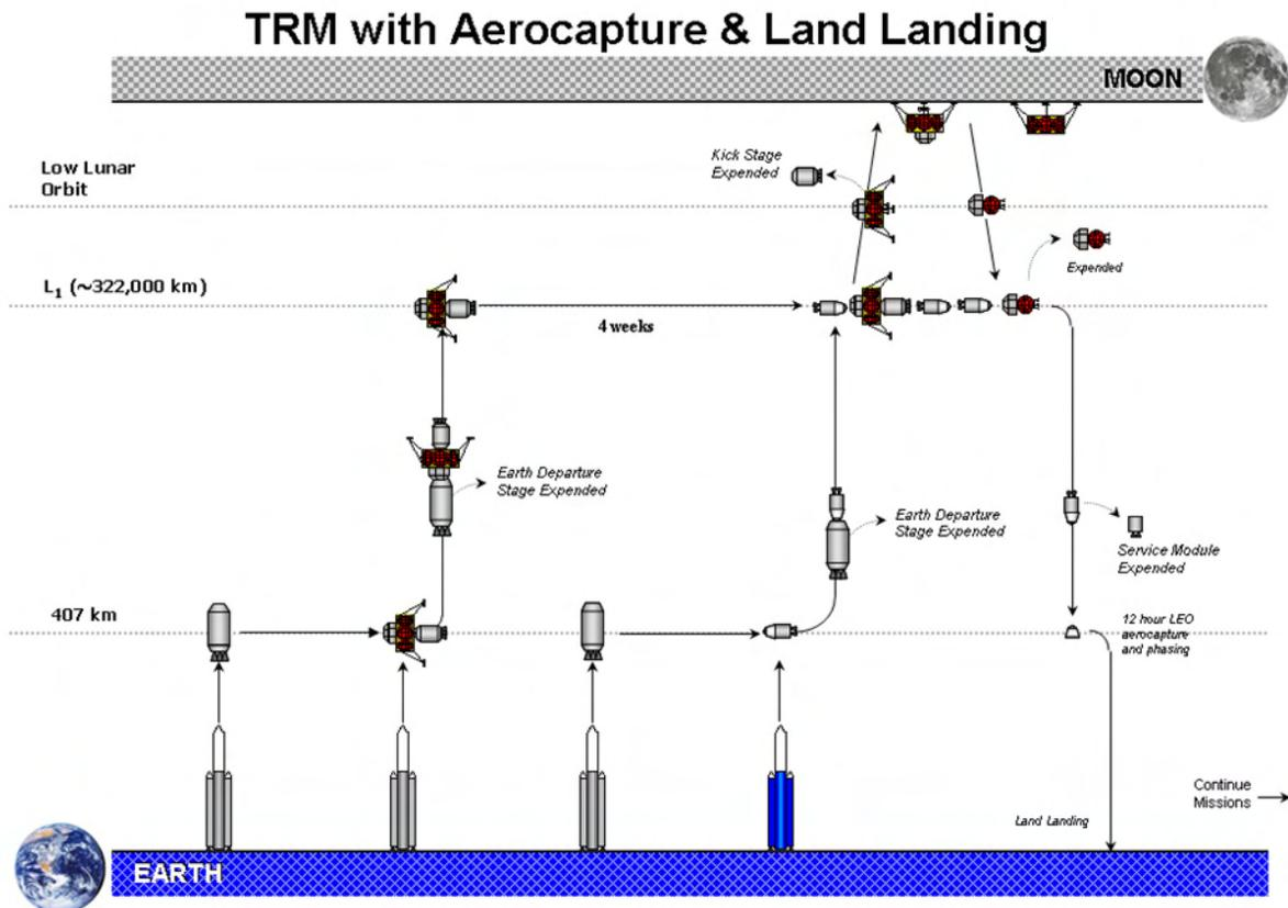
Figure 16.2-1: Aerocapture, Phasing, and Land-Landing Architecture Illustration
