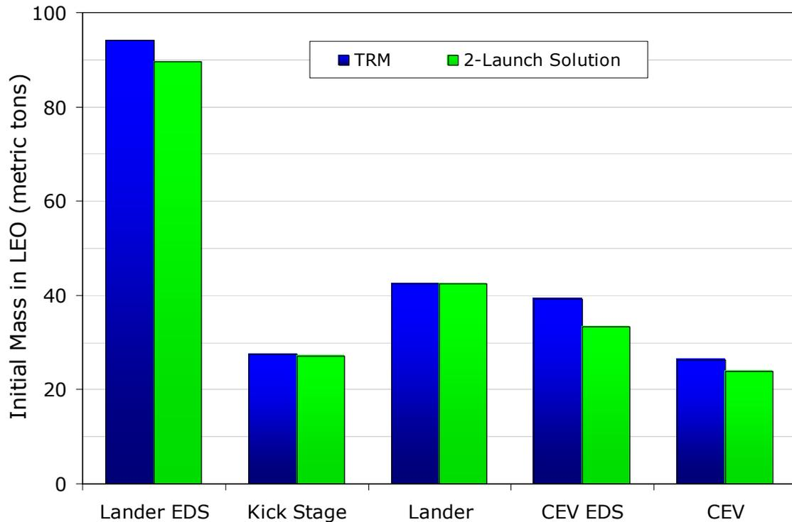
**Figure 11.5.5-1: Vehicle Mass Properties Comparison**
