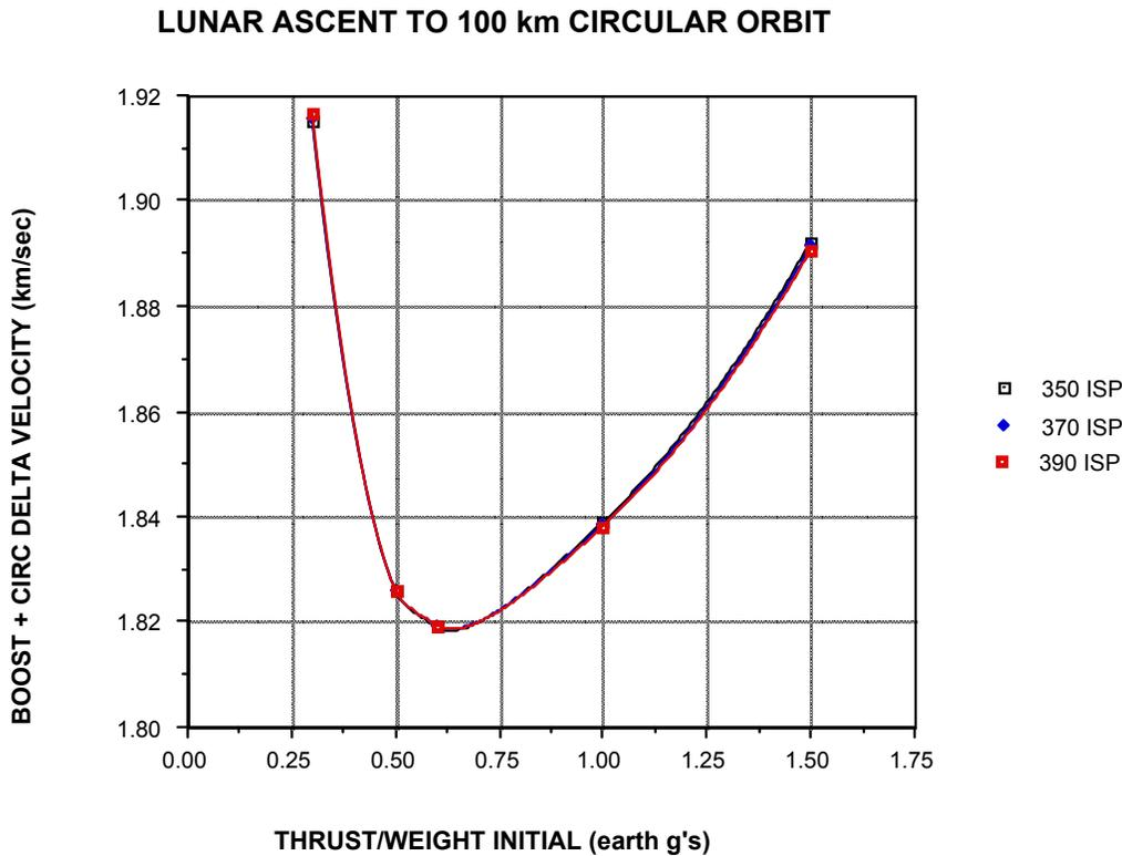
**Figure 10.5.2-1: Ascent Delta-V as a Function of Initial Thrust-to-Weight**
