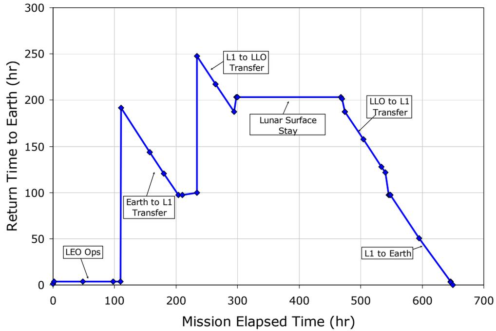
Figure 10.4.4-1: Maximum Return Time to Earth for TRM
