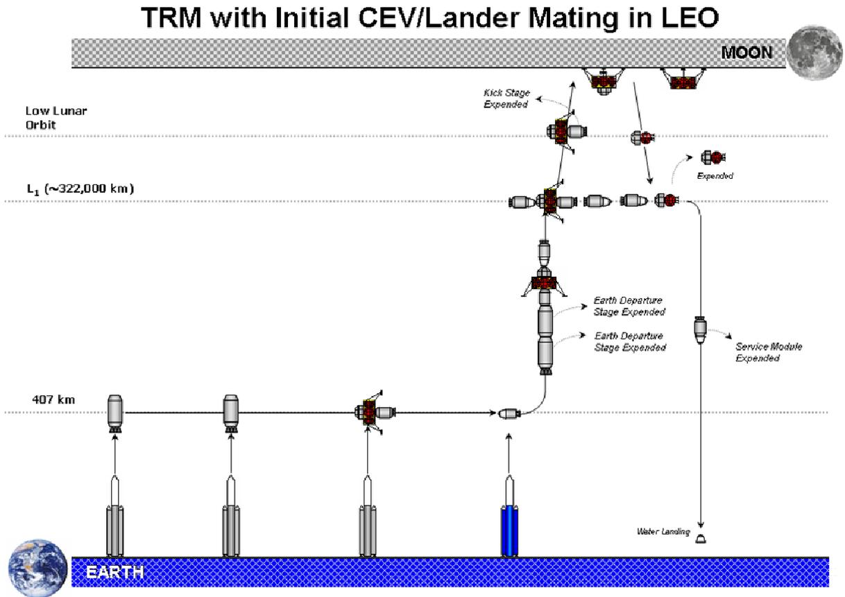
**Figure 15.2-1: Earth Orbit Rendezvous Architecture Illustration**
