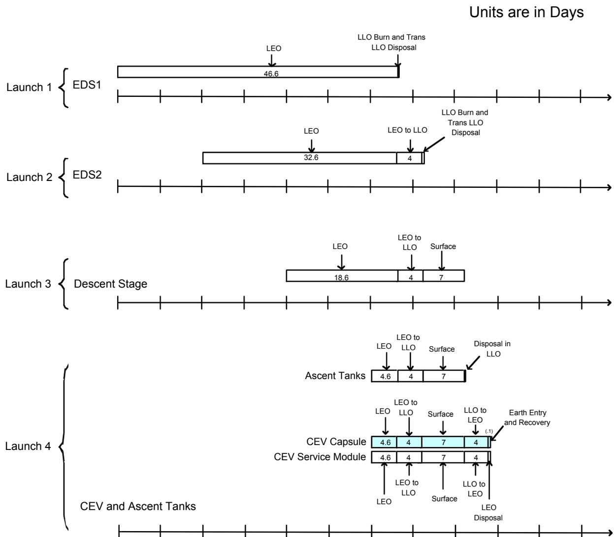
**Figure 17.2-2: Nominal Mission Timeline for the Direct Return Architecture**
