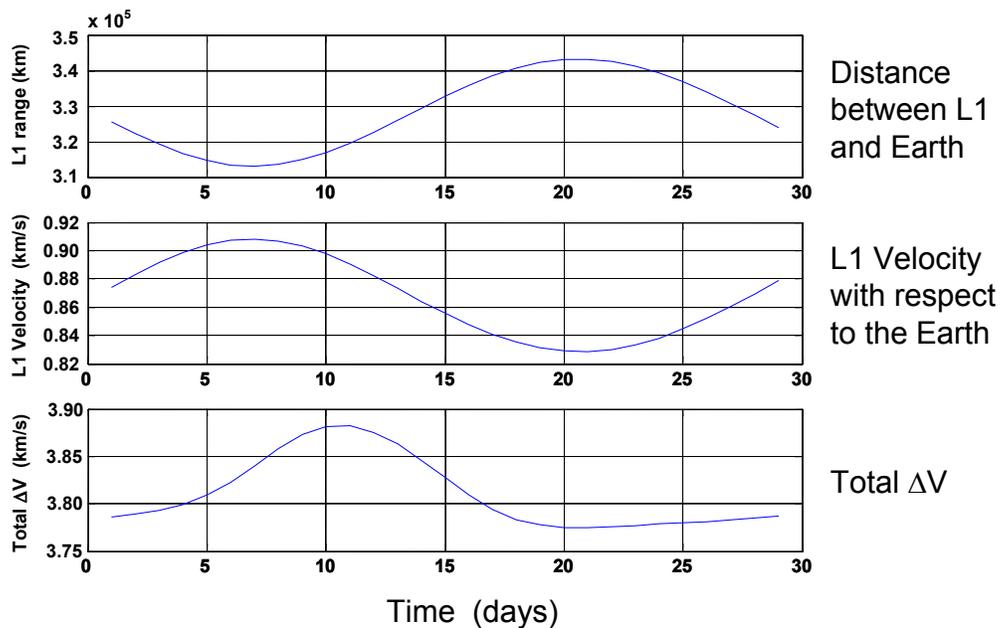
**Figure 8.2.5-3: Total  $\Delta V$  after 28 days (bottom figure) and L1 distance and velocity with respect to the Earth at arrival (top figure)**
