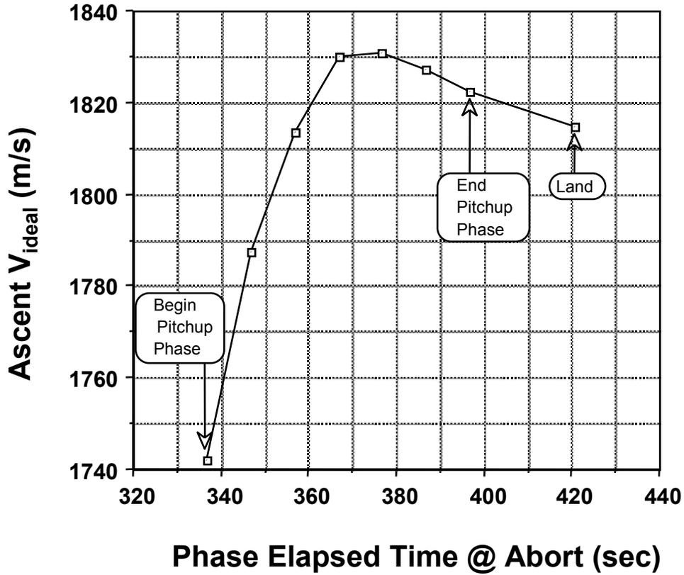
**Figure 8.2.7-6: Ascent ideal velocity versus phase elapsed time from the beginning of the pitchup/throttledown phase to touchdown (Abort from touchdown is the same as a nominal ascent)**
