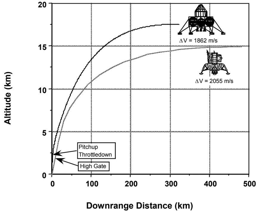
**Figure 8.2.7-3: FLO lander and Apollo LM altitude versus downrange distance for the powered descent to the lunar surface**
