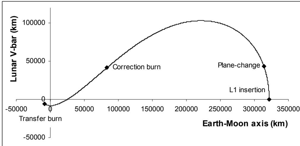
**Figure 8.2.5.2-1: LEO to L1 Transfer Trajectory**
