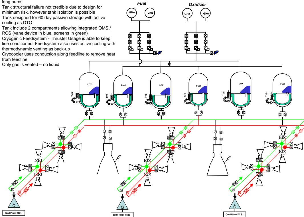
**Figure 19.1.1.3-2: CEV SM Propulsion Schematic**
