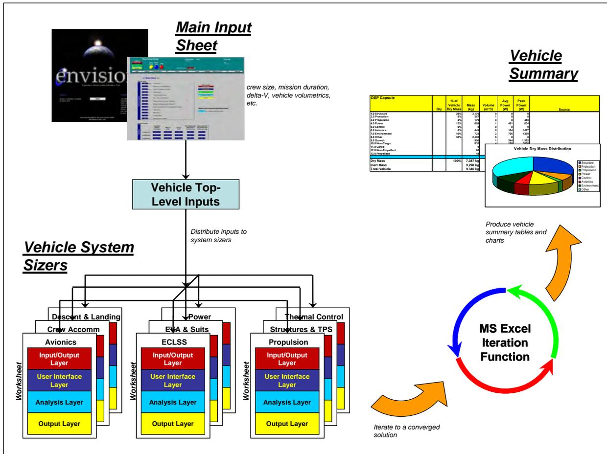
Figure 6.2-1: Envision Configuration Diagram
