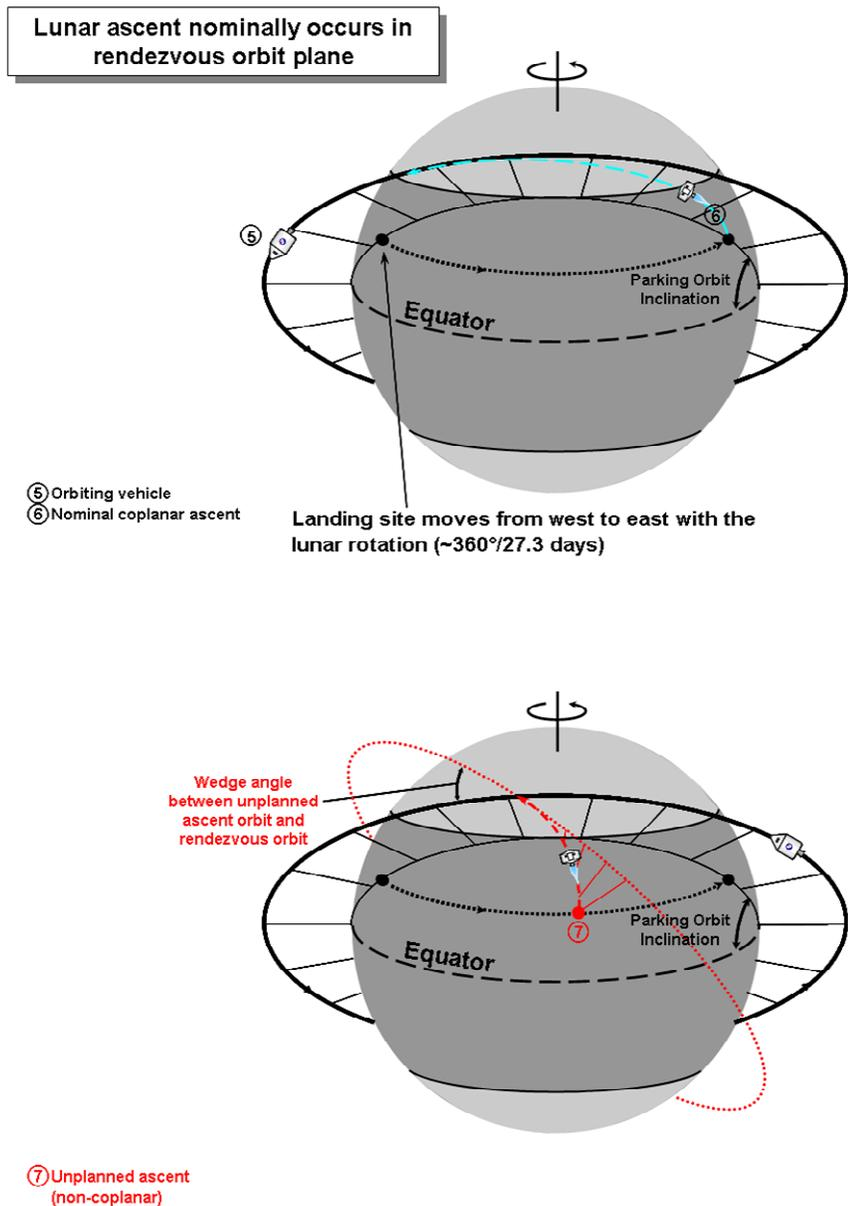
**Figure 14.2-1: Tailoring the Parking Orbit for Short-Stay LOR**
