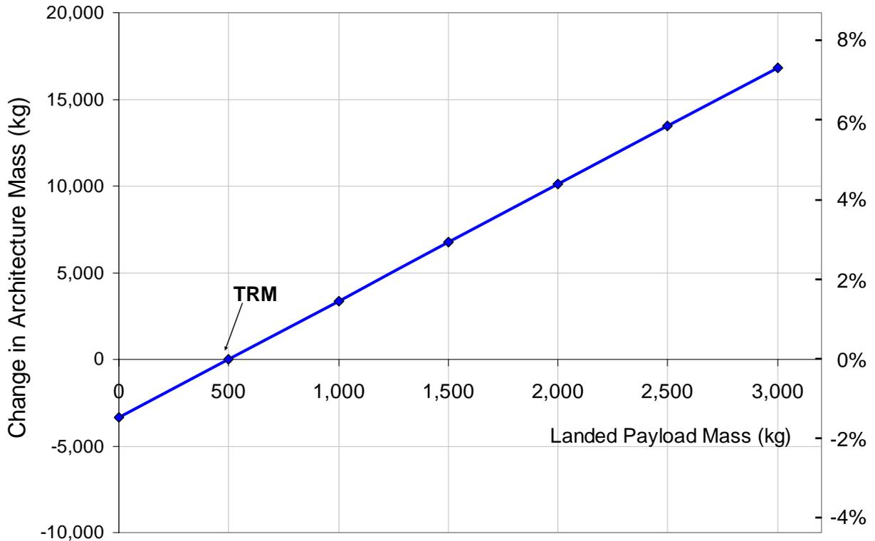
**Figure 19.4.2-1: Variation in Total Architecture Mass with Landed Payload Mass**
