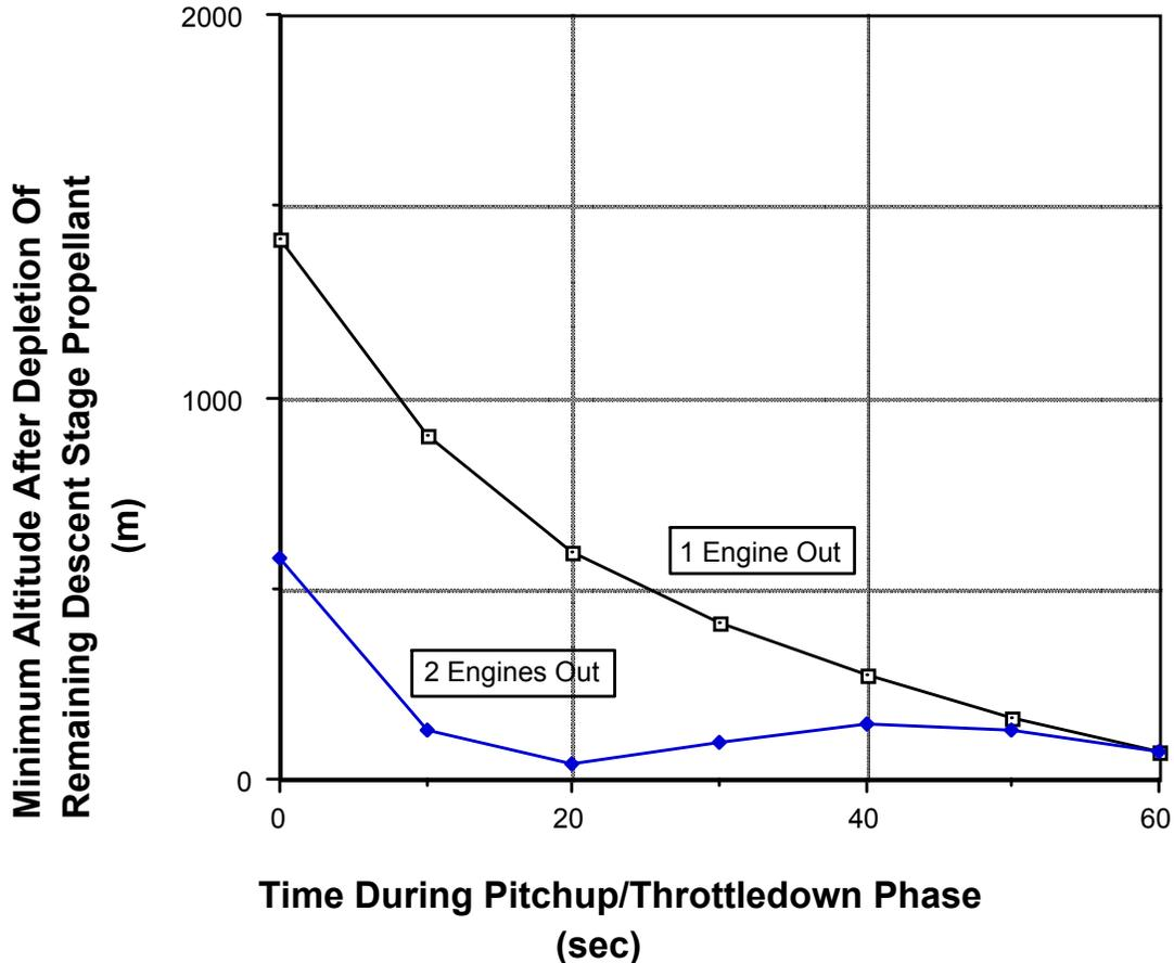
**Figure 8.2.7-12: Minimum altitude encountered versus time during the 60 second pitchup/throttledown phase for a one and two engine out descent stage assisted ascent to orbit**
