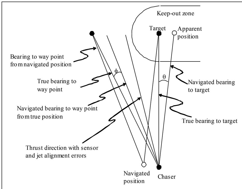
**Figure 8.2.5.2-5: Errors impacting bearing to way point (not to scale)**
