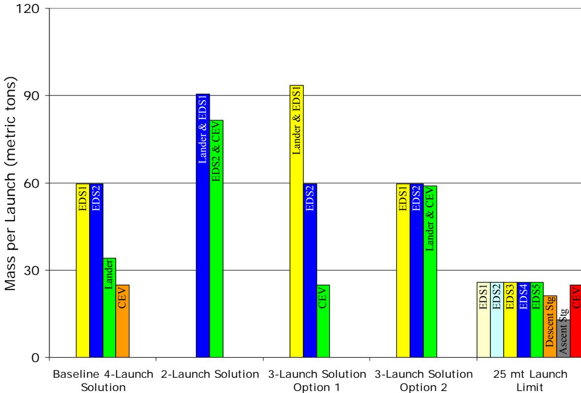
**Figure 7.4-4: Launch Requirements for Polar TRM Architecture Variants**
