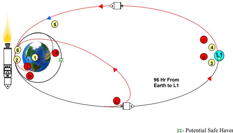
**Figure 9.2.2-1: Mission Abort Options for L1 CEV Dormant Architecture**
