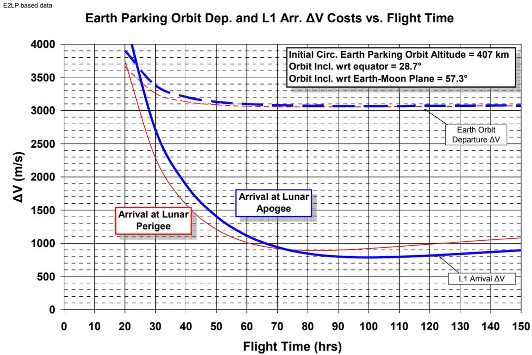
Figure 8.2.4.1-1: Earth Departure and L1 Insertion  $\Delta V$
