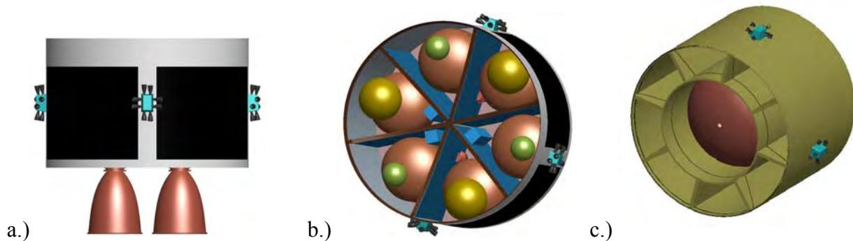
**Figure 20.1.2.4-3: a) Side View of SM, b) Six-Tank Configuration, c) Single Common Bulkhead Tank**
