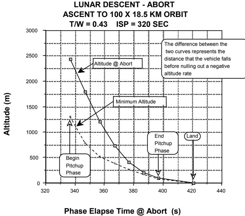
**Figure 8.2.7-7: Descent abort altitude and minimum altitude during ascent to orbit versus phase elapsed time during the powered descent**
