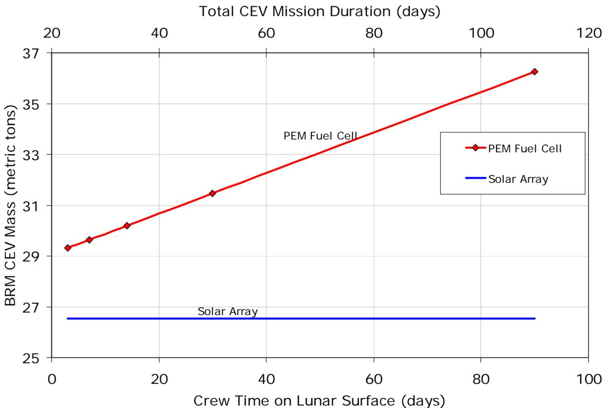
**Figure 19.2.2-1: Variation in CEV Mass with Power Technology and Lunar Stay Time**
