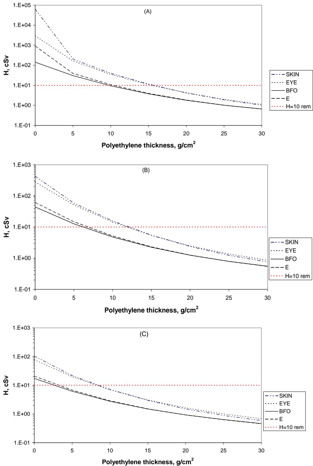
**Figure 20.15.3-2: Dose equivalent at sensitive sites from August 1972 SPE with various polyethylene shielding inside (A) 0, (B) 5, and (C) 10  $g/cm^2$  of aluminum**
