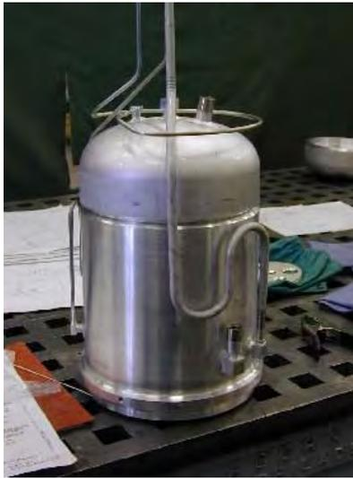
**Figure 20.1.2.3-1: Common Bulkhead LO2 / LCH4 Tank**
