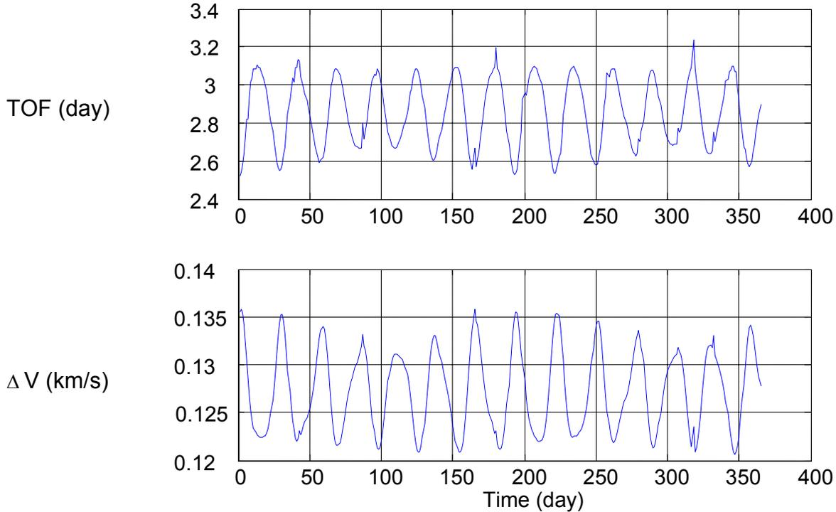
**Figure 8.2.8-5: Time of flight (TOF) and  $\Delta V$  for the stage disposal to the Moon in the year 2018**
