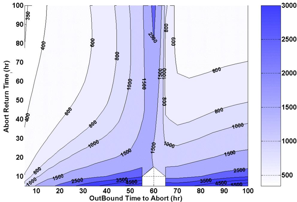
**Figure 8.2.6-4: Contour Plot of Total Abort  $\Delta V$**
