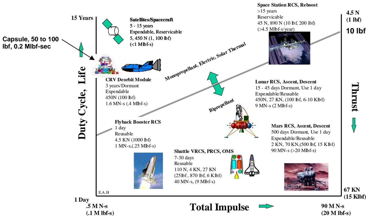
**Figure 19.1-1: Duty Cycle – Thrust – Total Impulse Considerations**
