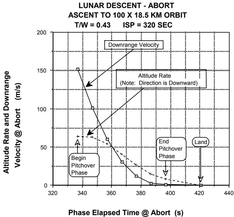
**Figure 8.2.7-8: Altitude rate and downrange velocity versus phase elapsed time during the powered descent**
