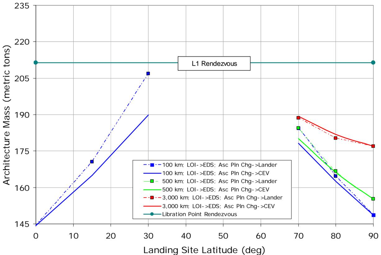
**Figure 7.2.1-1: Vehicle Sizing Results for Polar LOR Trade Options**
