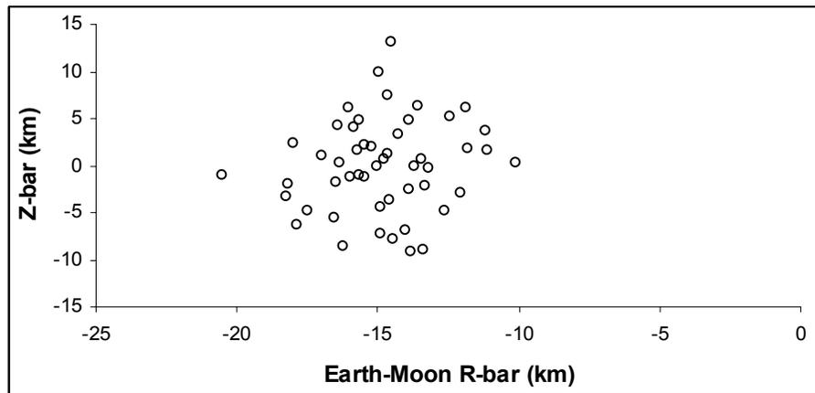
**Figure 8.2.5.2-3: Dispersions with Failure after Plane Insertion Burn**
