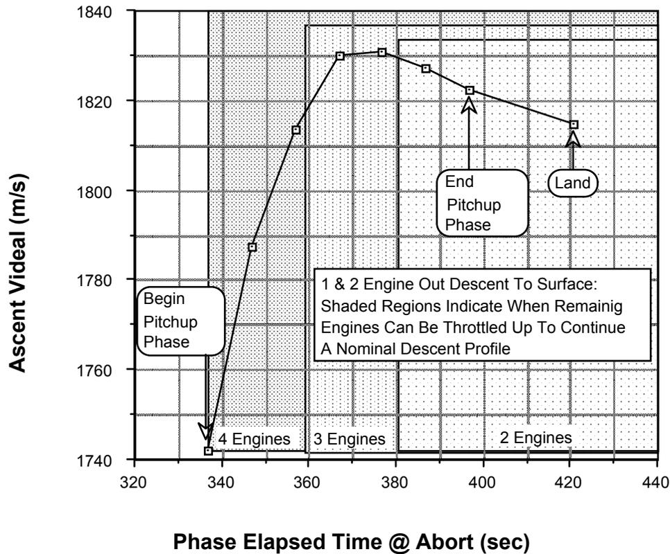
**Figure 8.2.7-13: Minimum altitude encountered versus time during the 60 second pitchup/throttledown phase for a one and two engine out descent stage assisted ascent to orbit**
