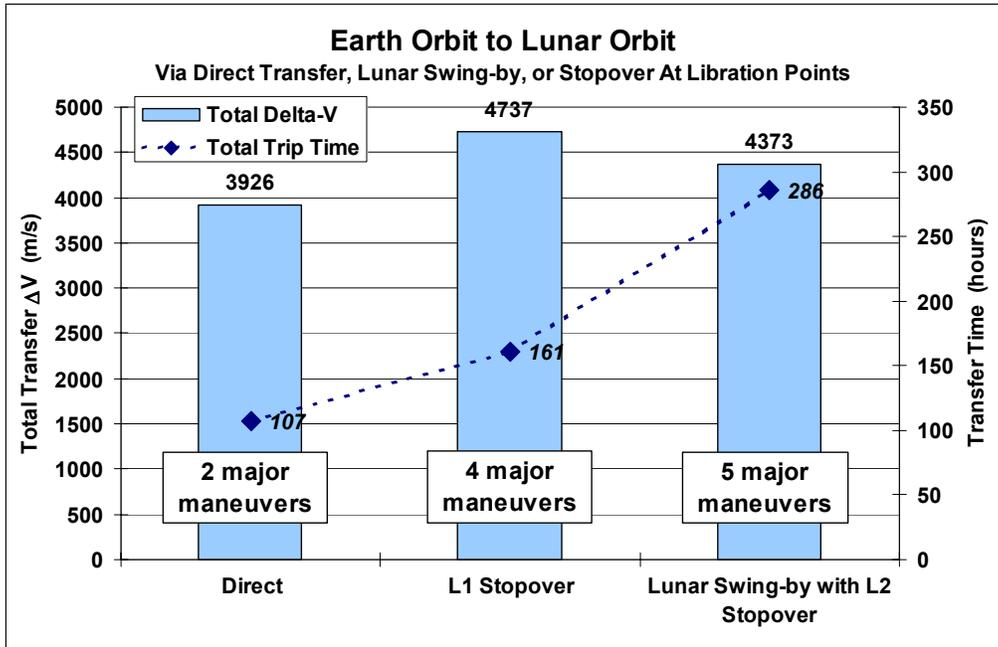
**Figure 8.1.2-1:  $\Delta V$ , Trip Time Comparison Of Earth-Moon Transfers Employing Either A Direct Transfer From Earth To The Moon Or One Including A Stopover At One Of The Collinear Earth-Moon Libration Points (L1, L2)**
