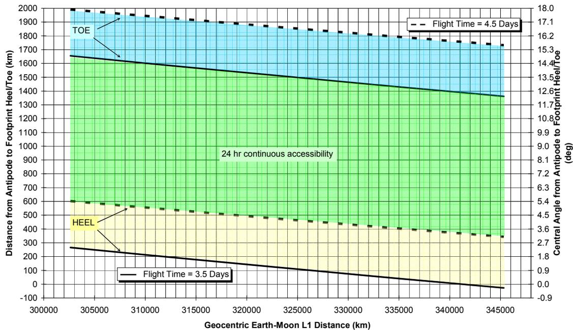
**Figure 8.2.9-6: Effective Apollo Footprint with respect to L1 Distance**
