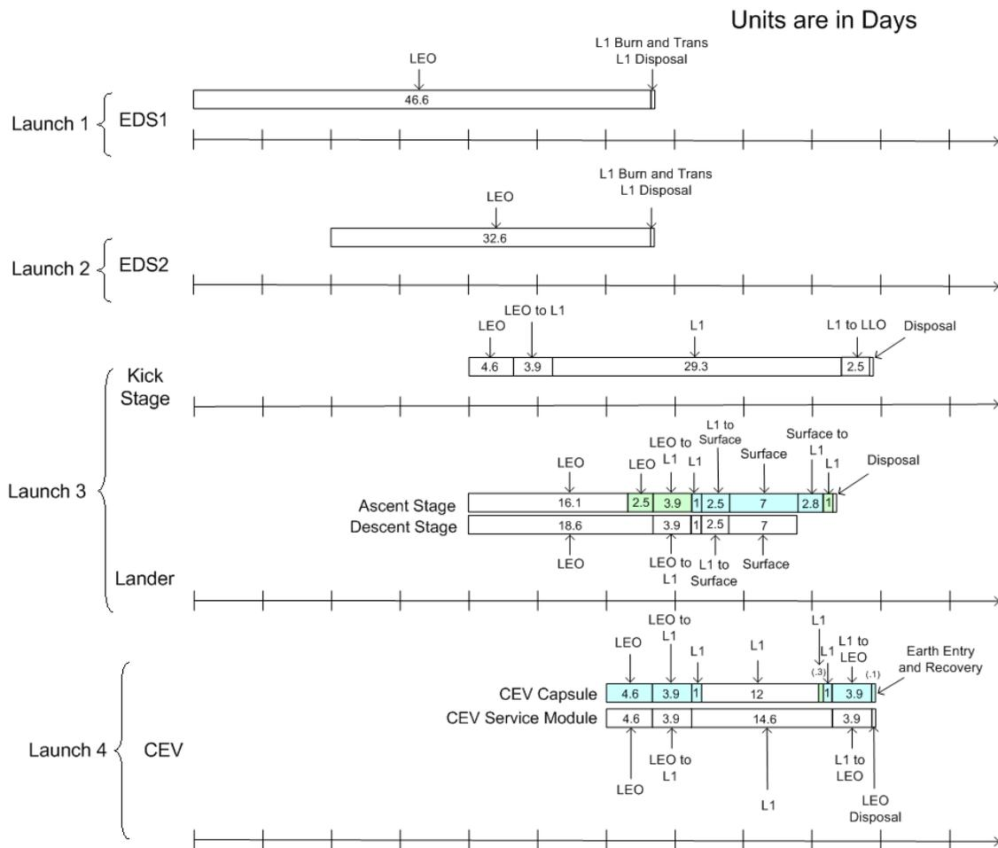
Figure 15.2-2: Nominal Timeline for the Earth Orbit Rendezvous Architecture
