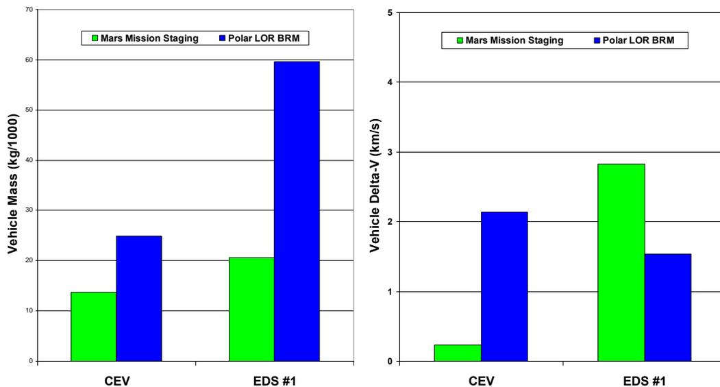
**Figure 11.3-1: CEV/EDS Mass and Delta V Comparison Between the LDRM-2 Phase 2 TRM and Mars Mission Staging Missions**
