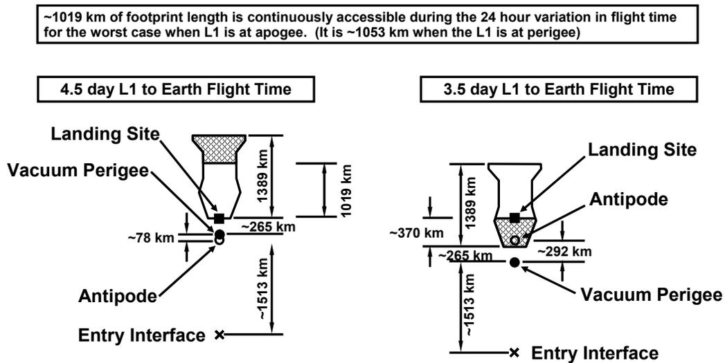
Figure 8.2.9-5: Effective Apollo Footprint for a 24 Hour Flight Time Variation
