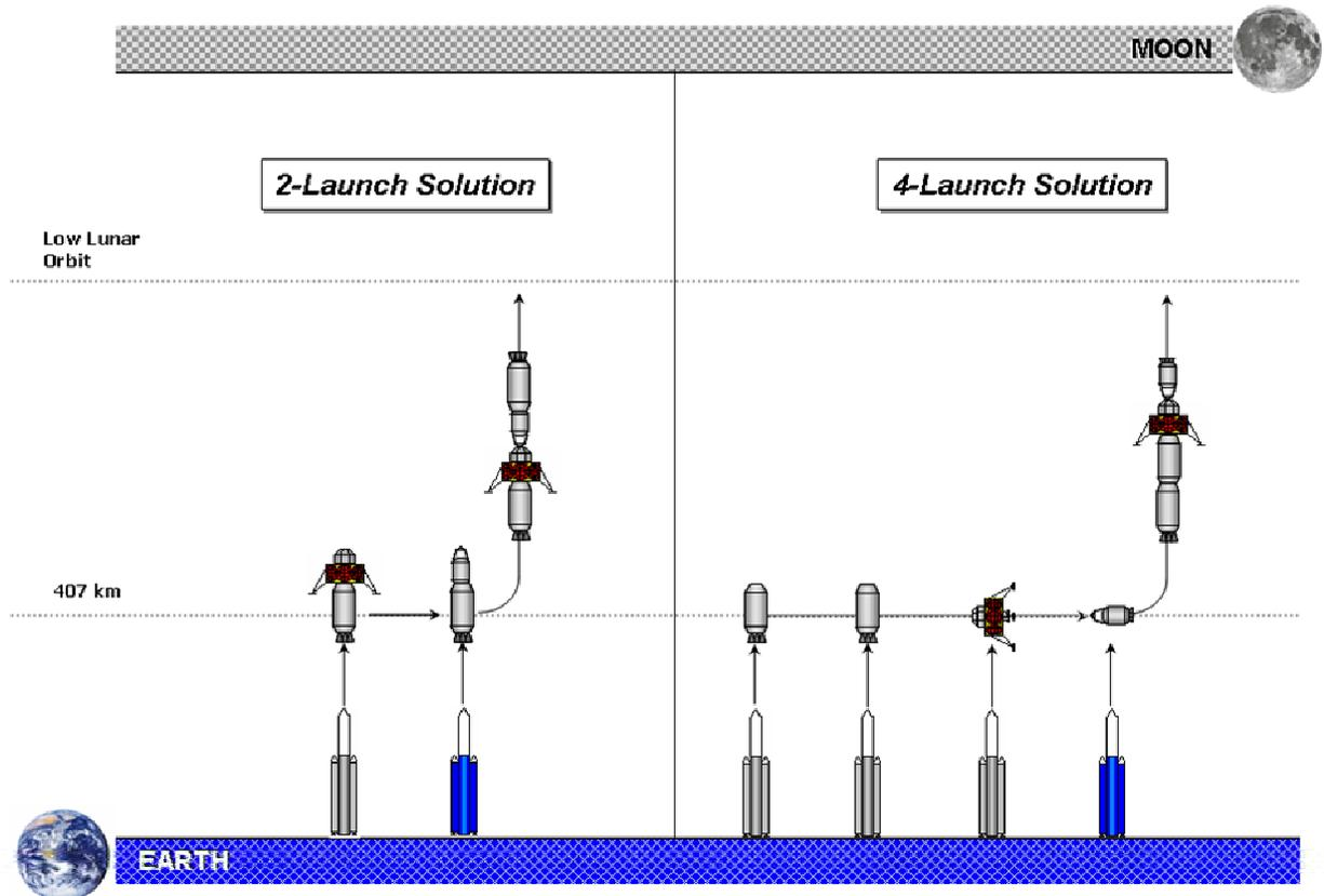
**Figure 7.4-1: Earth Orbit Departure Stack Configuration for 2-Launch Solution**
