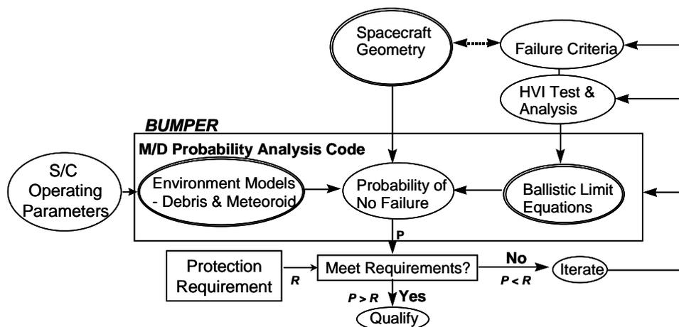
Figure 20.16.2-2: BUMPER Model Schematic
