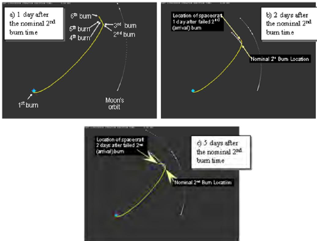
**Figure 8.2.5-4: Chaser and target trajectories after a failed 2nd burn**
