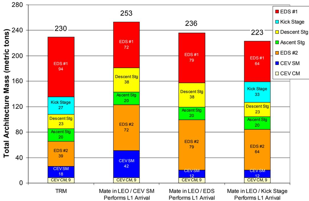
Figure 18.1.4-1: IMLEO for the L1 TRM and Tandem EOD Options
