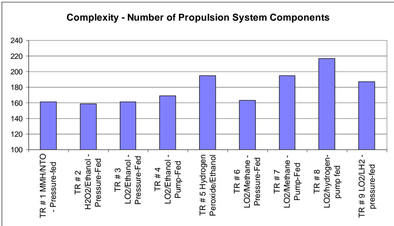
Figure 19.1.1.1-3: Complexity – Number of Components
