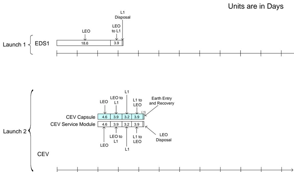
**Figure 10.2.1-2: L1 CEV Active Architecture Nominal Timeline**
