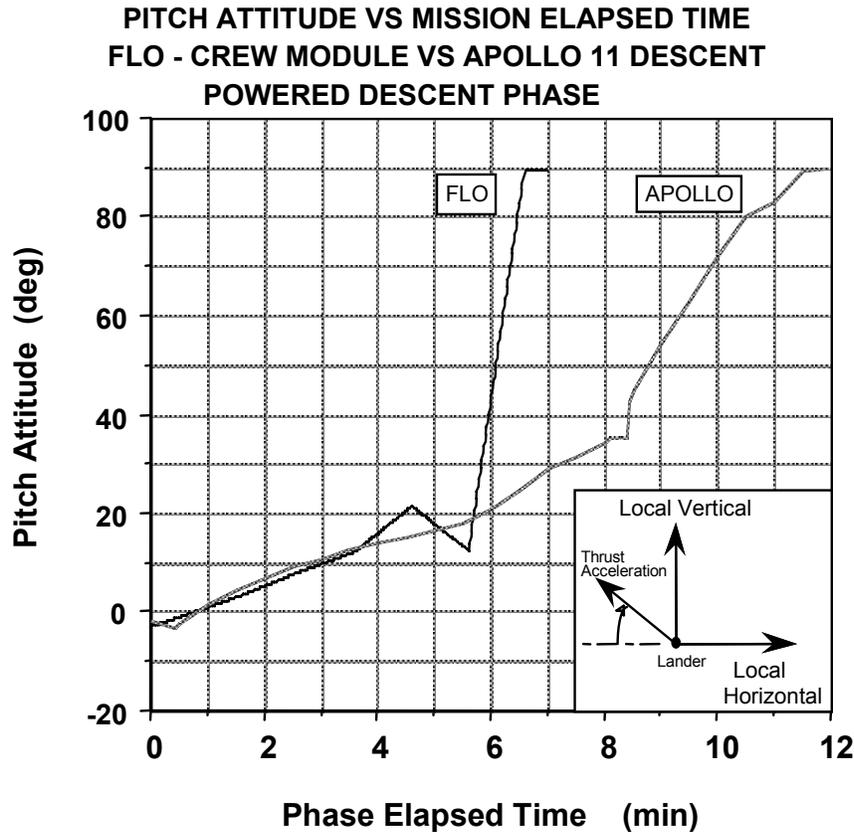
**Figure 8.2.7-4: FLO lander and Apollo LM pitch attitude versus phase elapsed time for the powered descent to the lunar surface**
