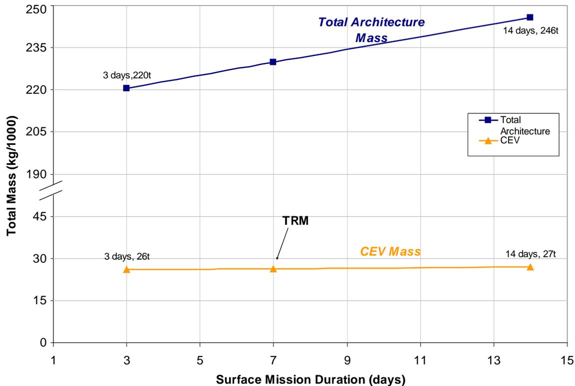
**Figure 19.9-1: Effects of Varying the Duration of the Surface Mission on Total Architecture Mass**
