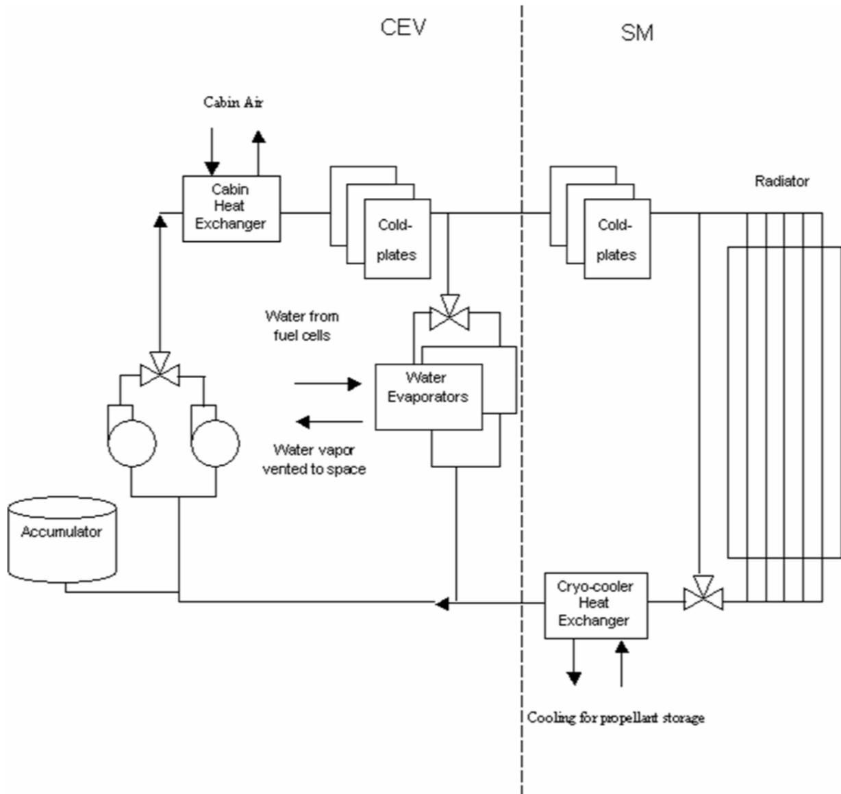
**Figure 20.5.3.1-1: CEV Command Module/Service Module ATCS Schematic**
