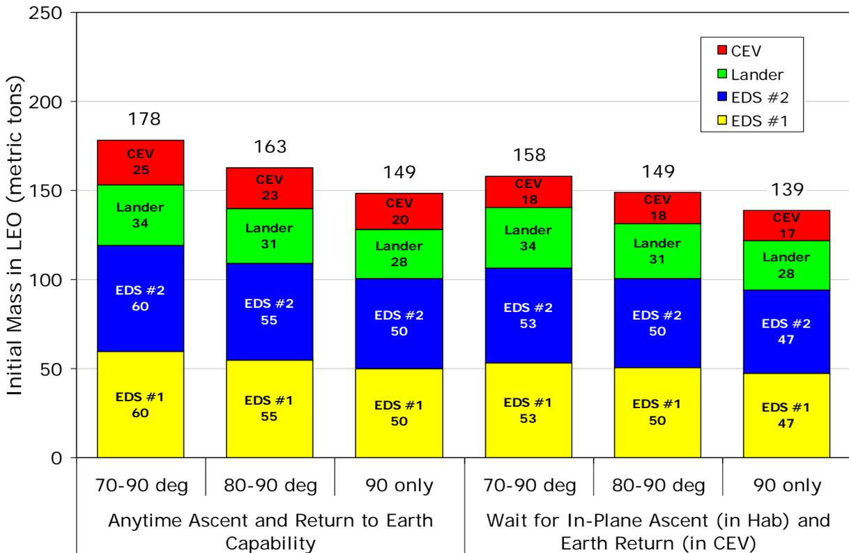
**Figure 7.5-3: Architecture Mass Cost of Anytime Ascent and Earth Return**
