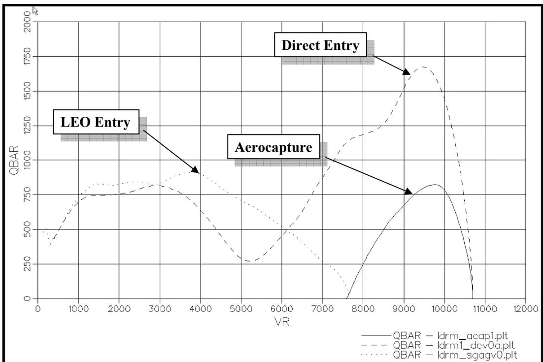
Figure 8.2.10-2: Dynamic Pressure (kg/m<sup>2</sup>) versus Relative Velocity (m/s)
