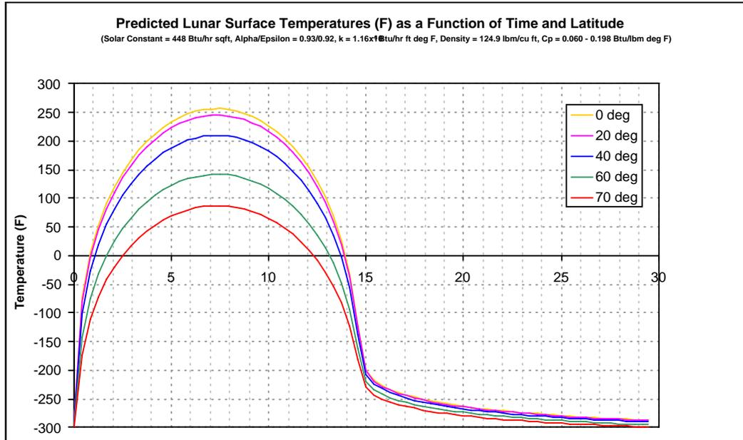
**Figure 20.14.5-1: Predicted Diurnal Lunar Surface Temperatures as a Function of Latitude**
