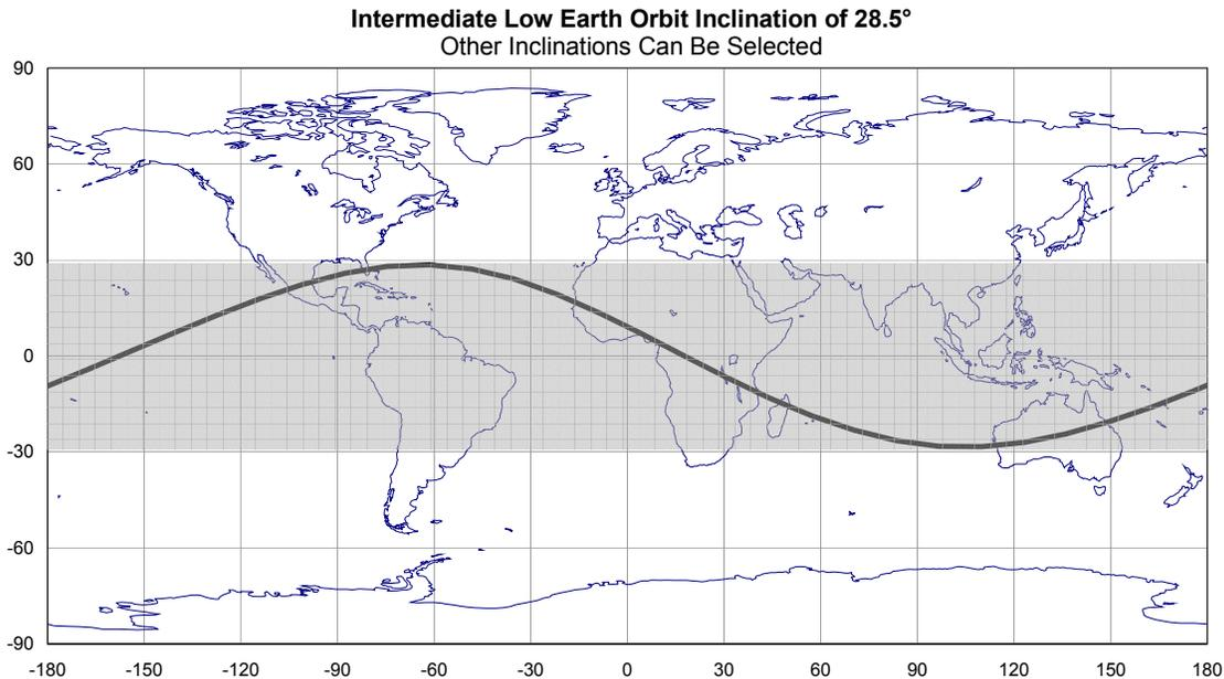
**Figure 16.2-3: Accessible Latitudes From a Fixed  $28.5^\circ$  Inclination**
