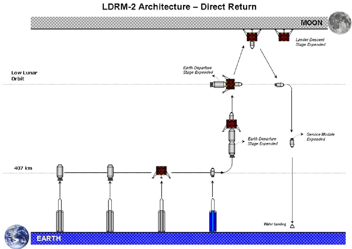
**Figure 17.2-1: Mission Flow of the TRM with Direct Return**
