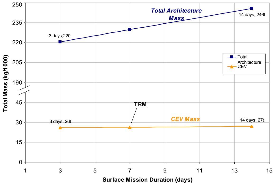
**Figure 19.10-1: Effects of Varying the Duration of the Surface Mission on Total Architecture Mass**
