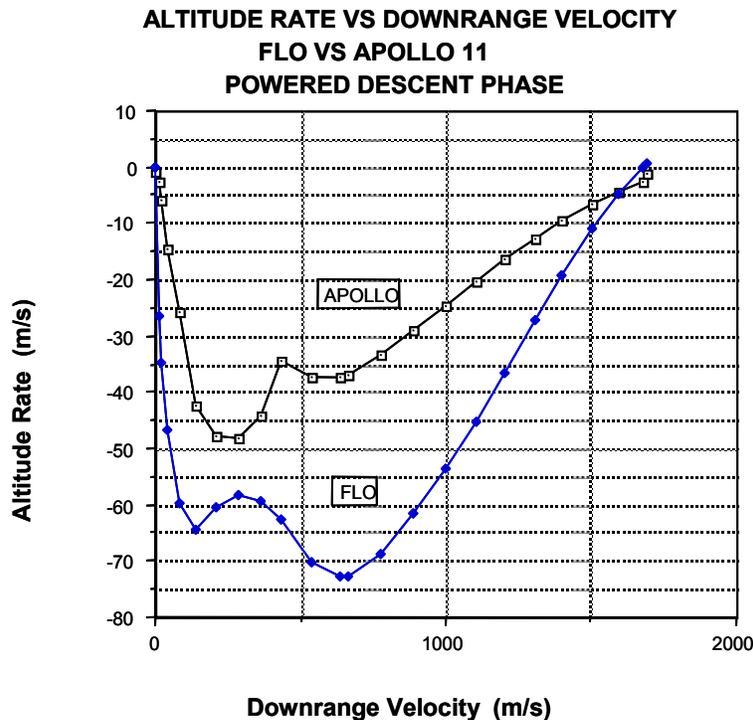
**Figure 8.2.7-9: Altitude rate versus downrange for Apollo and FLO landers**
