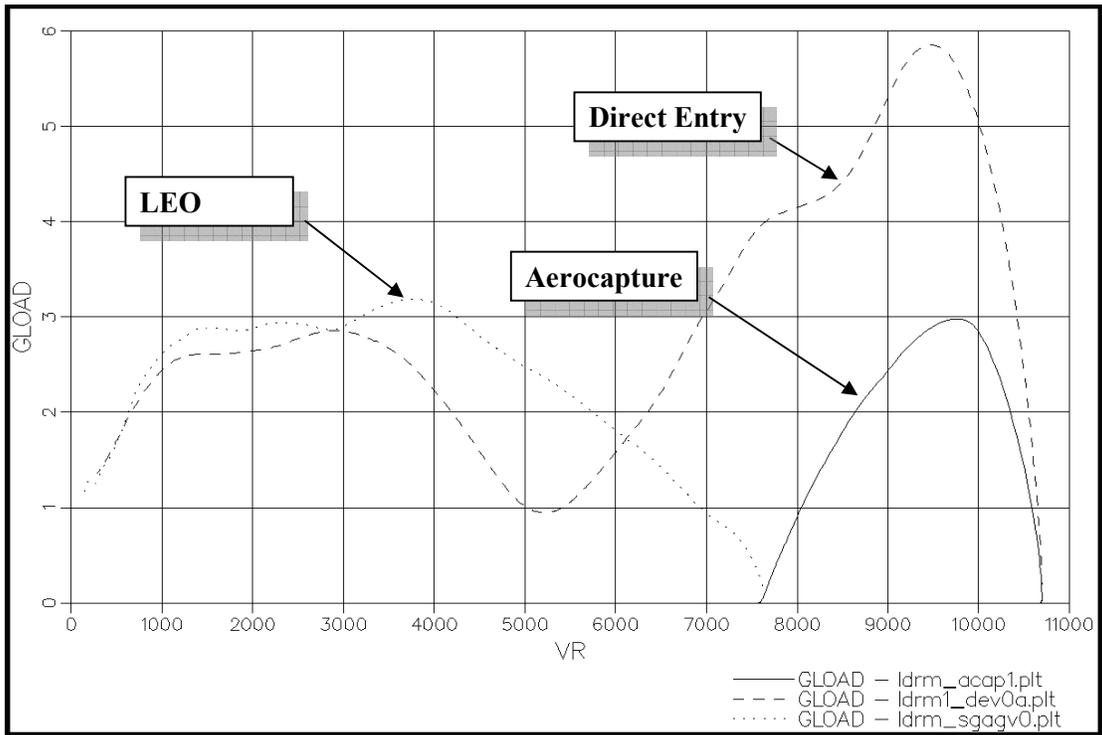
Figure 8.2.10-3: G-Load (Gs) versus Relative Velocity (m/s)
