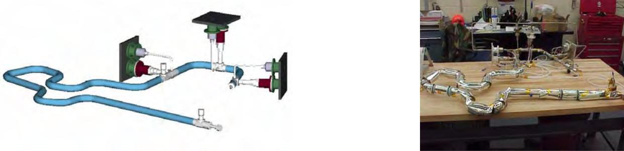
**Figure 20.1.2.3-2: RCS Feedsystem breadboard test article (outside of 8 ft vacuum chamber)**
