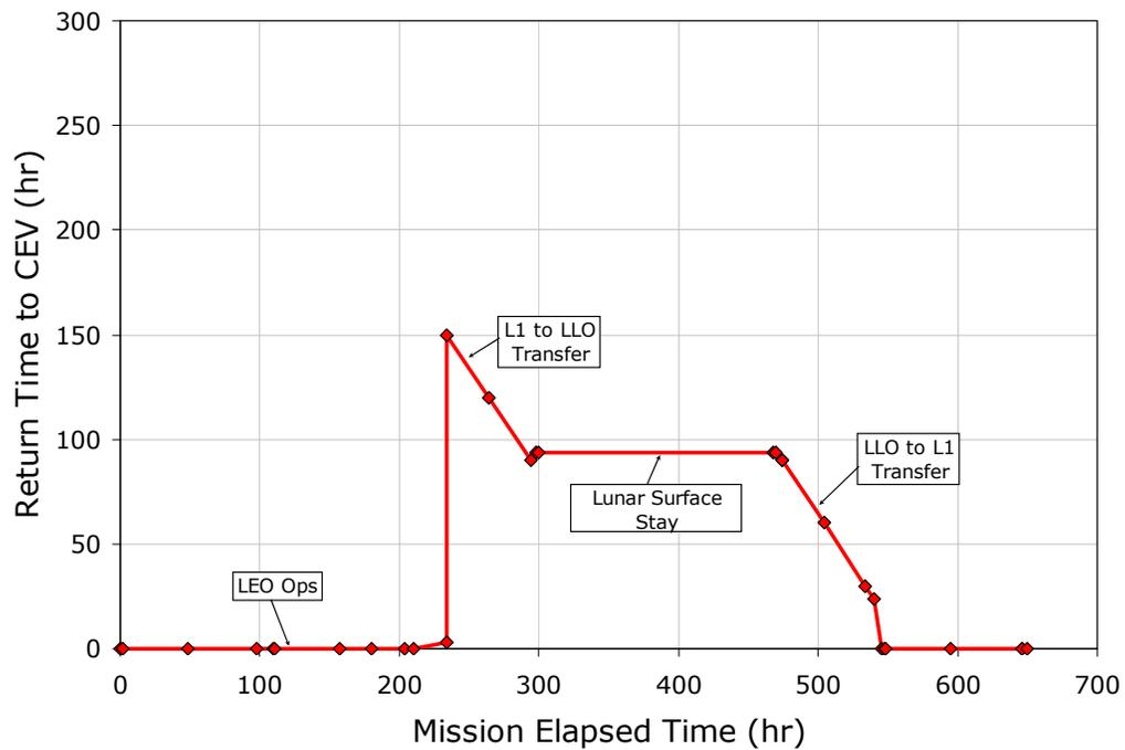
Figure 10.4.4-2: Maximum Return Time to CEV for TRM
