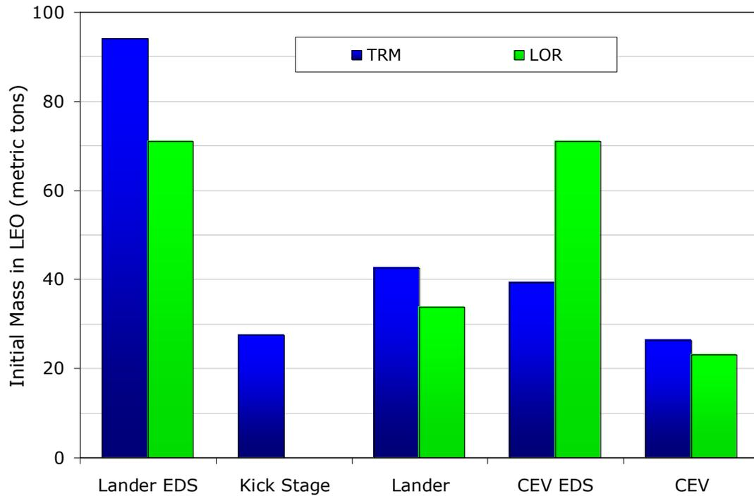
**Figure 14.5.5-1: Vehicle Mass Properties Comparison**
