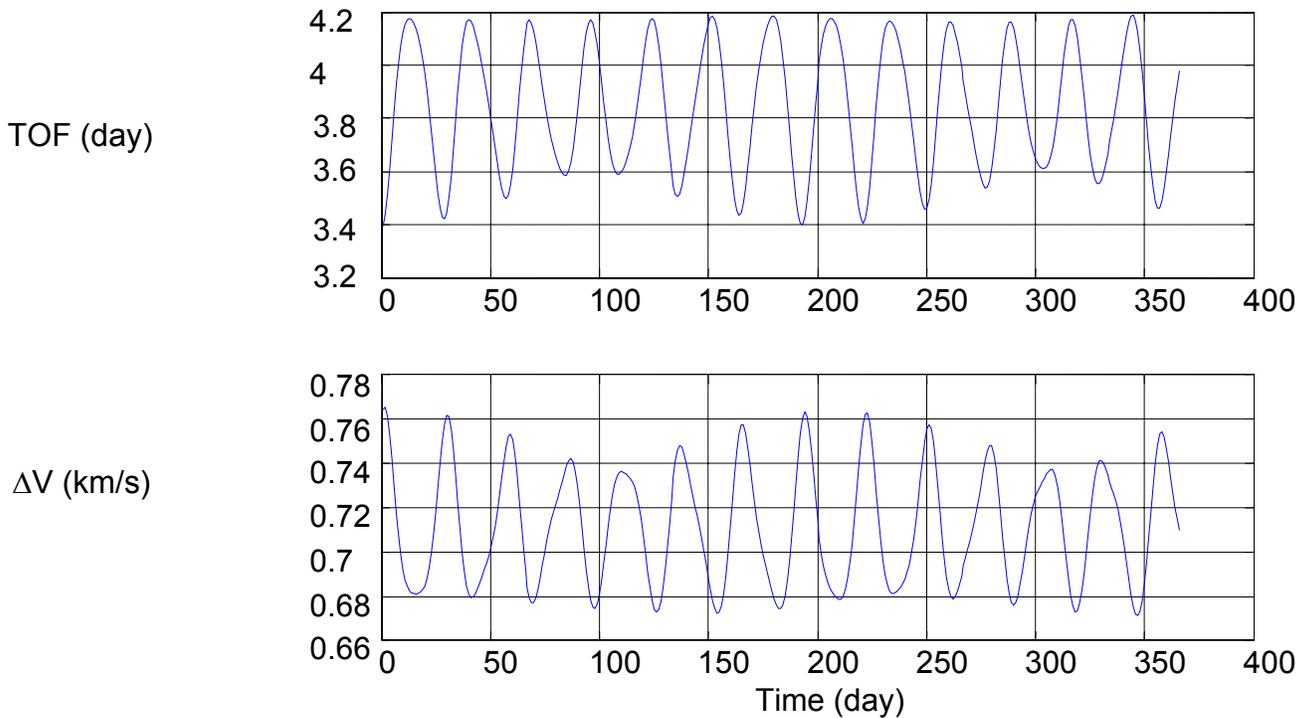
**Figure 8.2.8-3: Time of flight and  $\Delta V$  for the stage disposal to the Earth in the year 2018**
