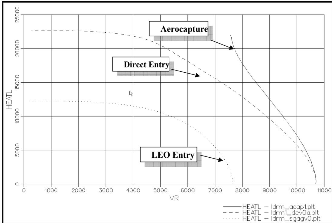
**Figure 8.2.10-5: Heat Load (J/cm<sup>2</sup>) versus Relative Velocity (m/s)**
