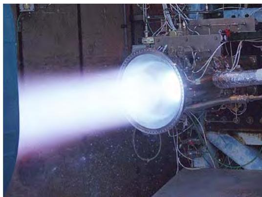
**Figure 20.1.2.3-3: 6000 lbf Unmodified Rocketdyne / DASA Aestus MMH/NTO Engine Running on Lox / Ethanol**
