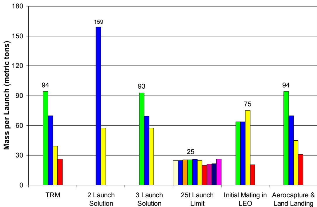
Figure 18.1-2: Mass per Launch for the L1 TRM and Architecture Variants
