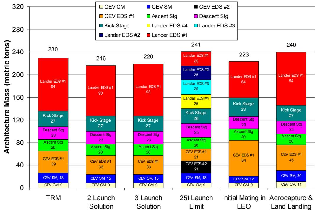
Figure 18.1-1: IMLEO for the L1 TRM and Architecture Variants
