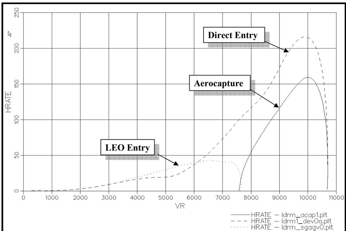
Figure 8.2.10-4: DKR Heat Rate (W/cm<sup>2</sup>) versus Relative Velocity (m/s)
