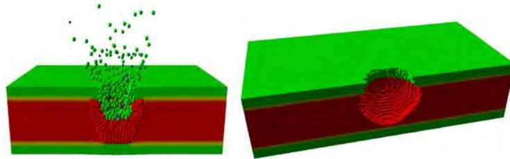
Hypervelocity impact and simulation results indicate that 1" of low-density SiC-foam behind the RCC panel or on WLE spar reduces meteoroid/debris penetration risk by factor of 20 from current single wall RCC design.
