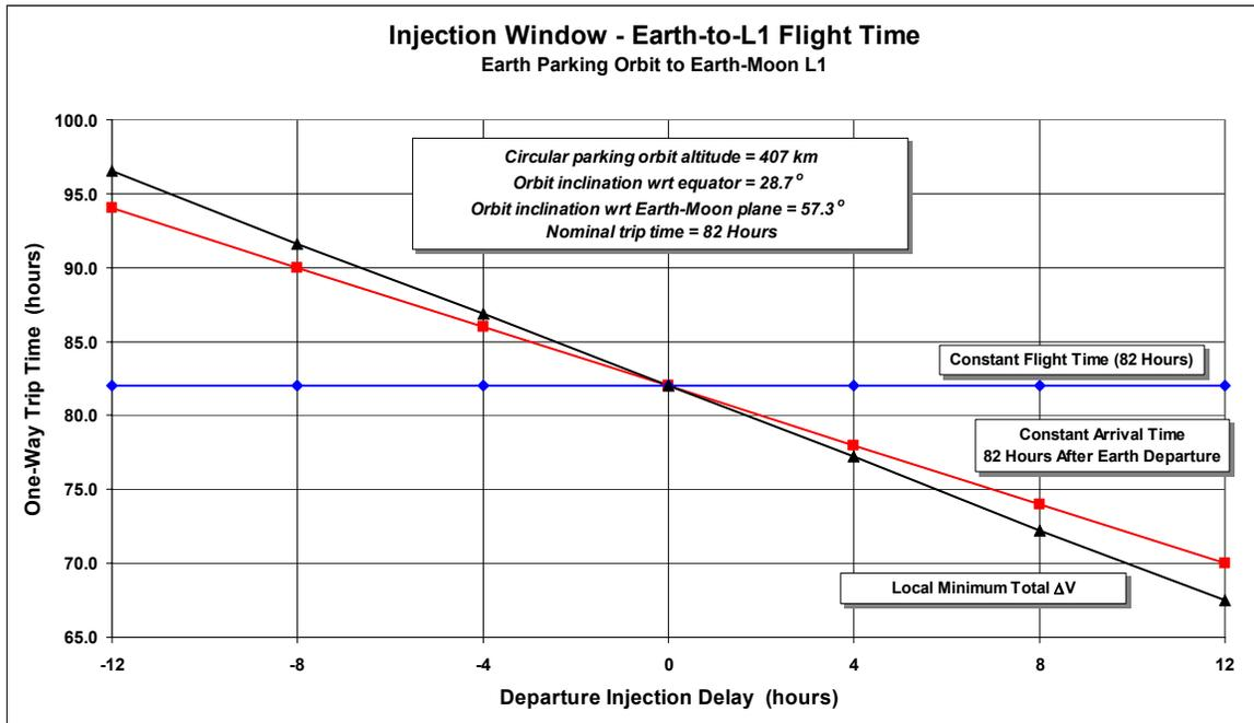
**Figure 8.2.1-1c: Flight Time Versus Earth Departure Time For A Twenty-Four (24) Hour Earth Departure Injection Window**
