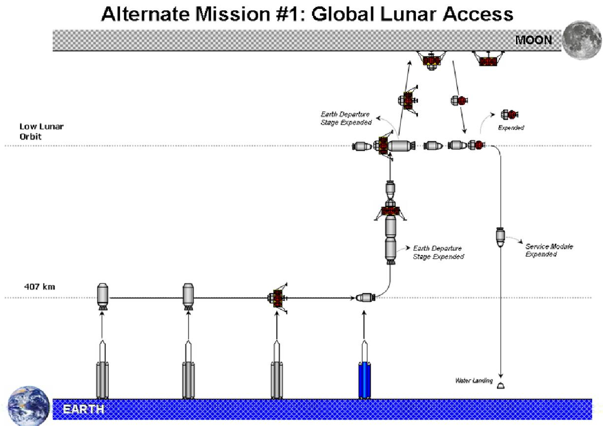
**Figure 8.2.1-1: Global Lunar Access Architecture Illustration**
