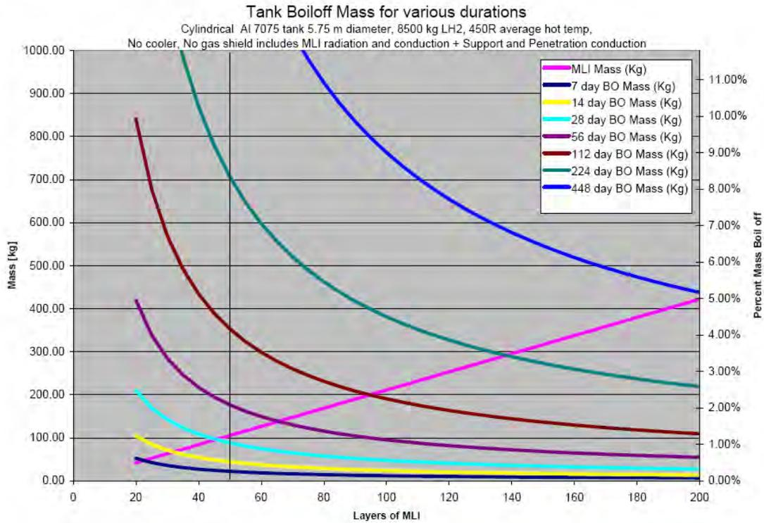
Figure 10.5.4-1: Hydrogen Boiloff for Earth Departure Stages
