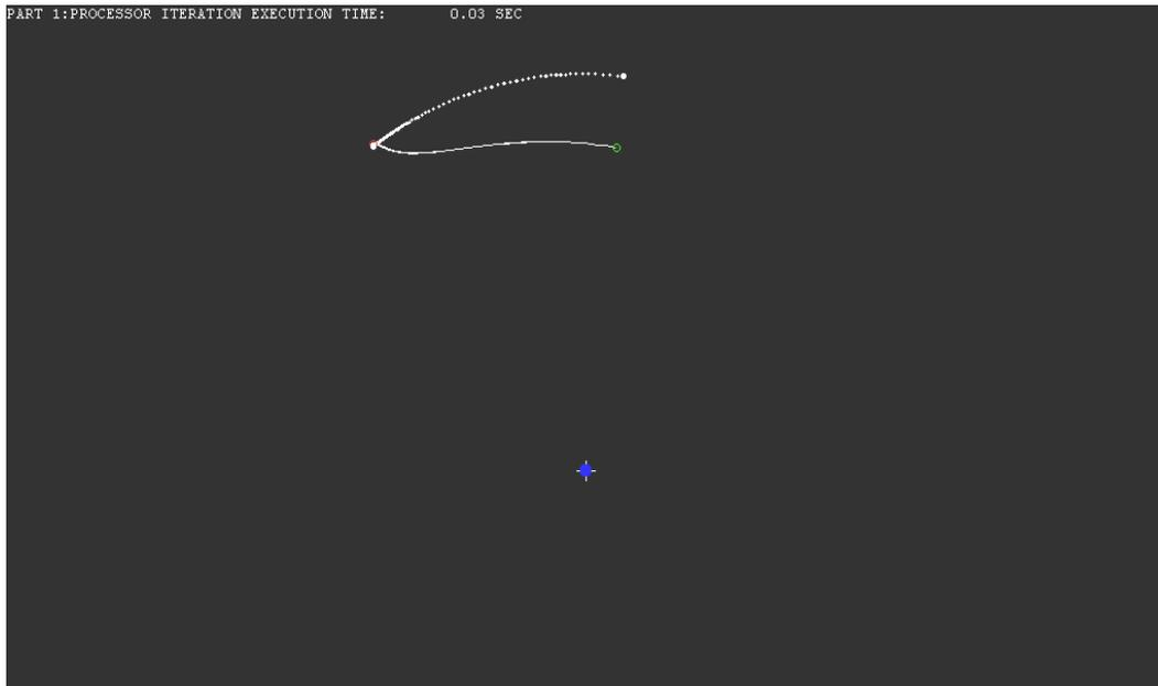
**Figure 8.2.8-4: Stage disposal trajectory to the Moon obtained with Copernicus. Transfer time = 2.6 days. Disposal maneuver  $\Delta V = 135$  m/s**
