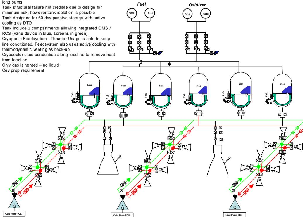
Figure 20.1.2.4-1: Integrated OMS/RCS Schematic
