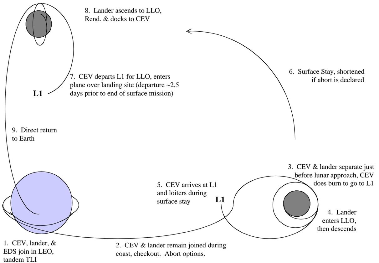
**Figure 7.3.1-1: Operations Concept for the Reference L1/LOR Hybrid Architecture**
