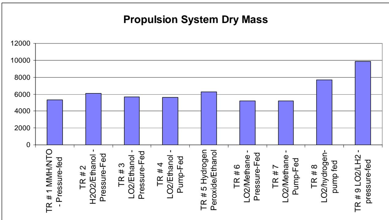
Figure 19.1.1.1-4: Propulsion System Dry Mass
