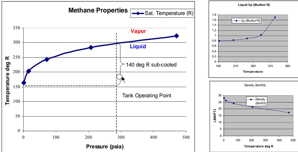
**Figure 20.1.2.4-2: Properties of Methane**
