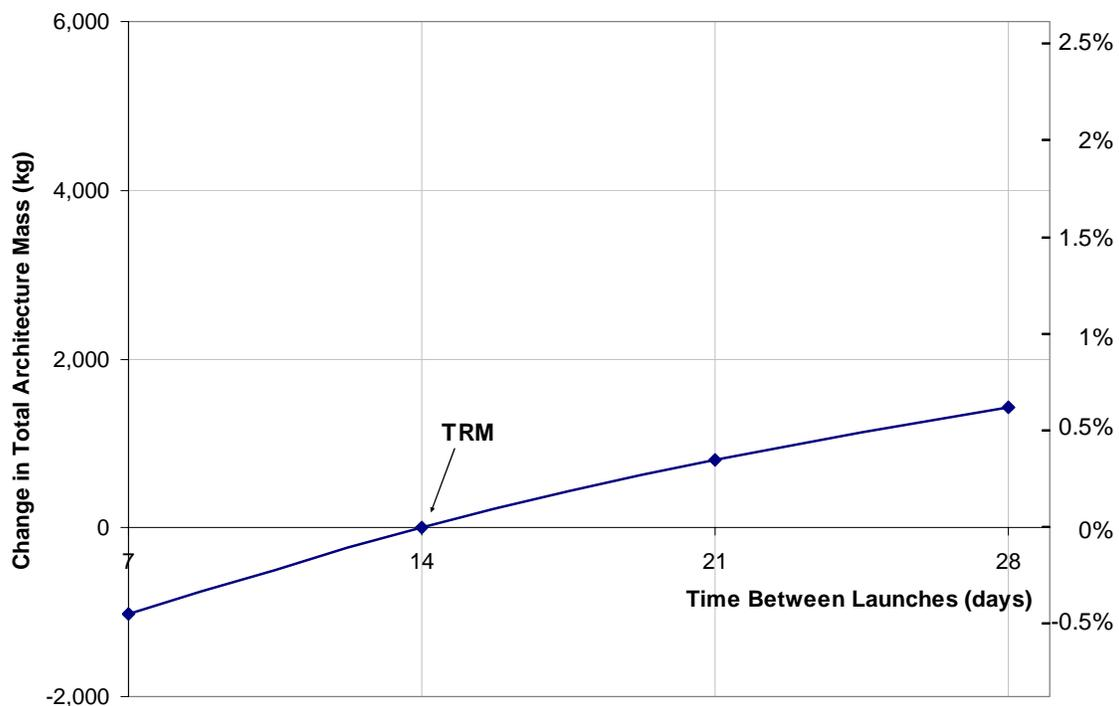
**Figure 19.8.1-1: Mass Impacts to Architecture from Varying Launch Interval**
