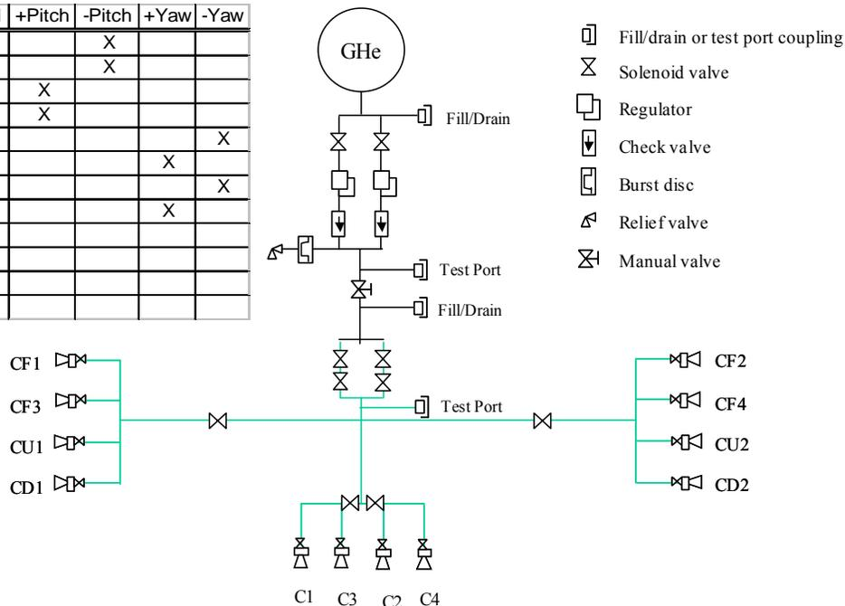
**Figure 20.1.1.3-1: CEV Entry Vehicle RCS Concept**
