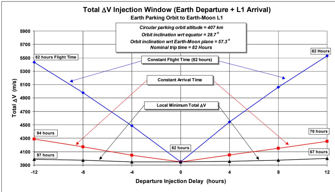
Figure 8.2.1-1a: Total  $\Delta V$  Cost Versus Earth Departure Time For A Twenty-Four (24) Hour Earth Departure Injection Window
