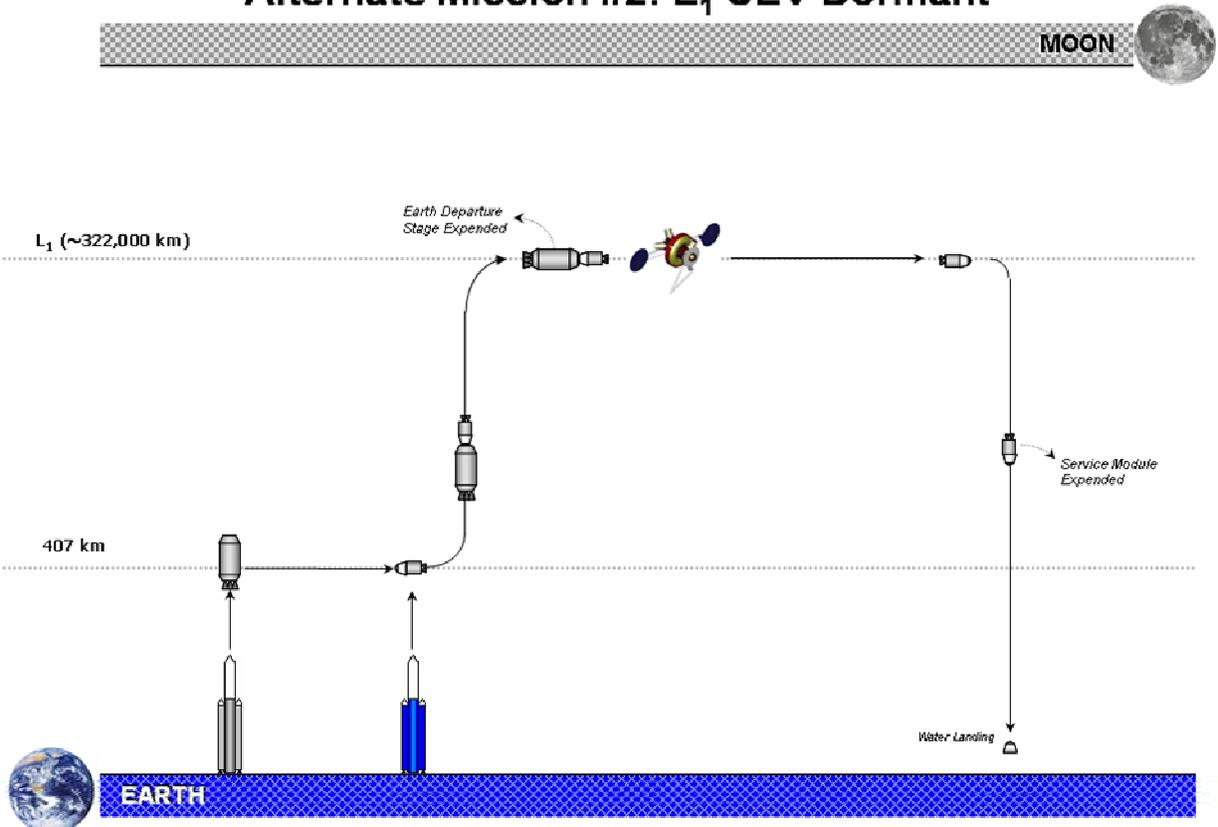
**Figure 9.2.1-1: L1 CEV Dormant Architecture Illustration**
