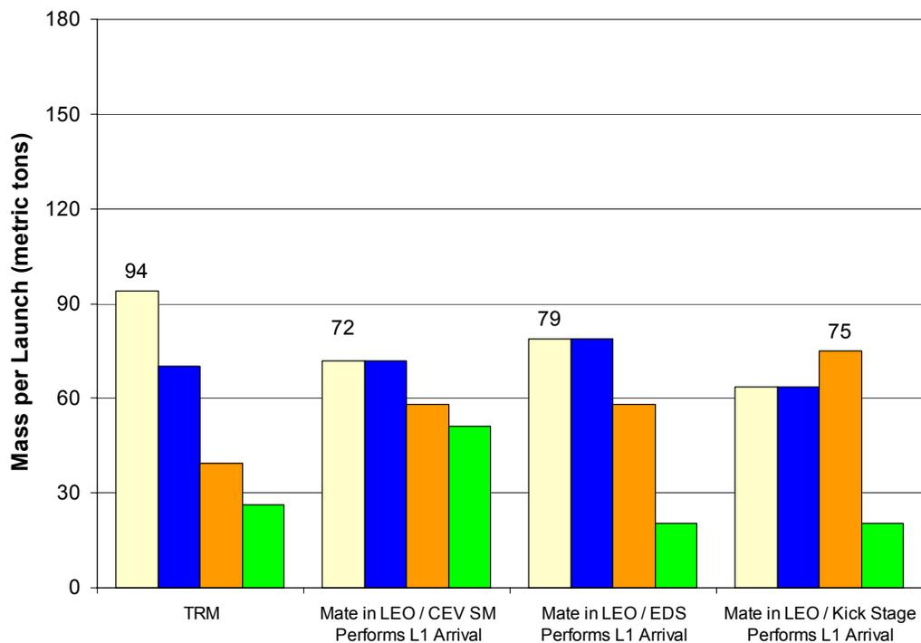
Figure 18.1.4-2: Mass per Launch for the L1 TRM and Tandem EOD Options
