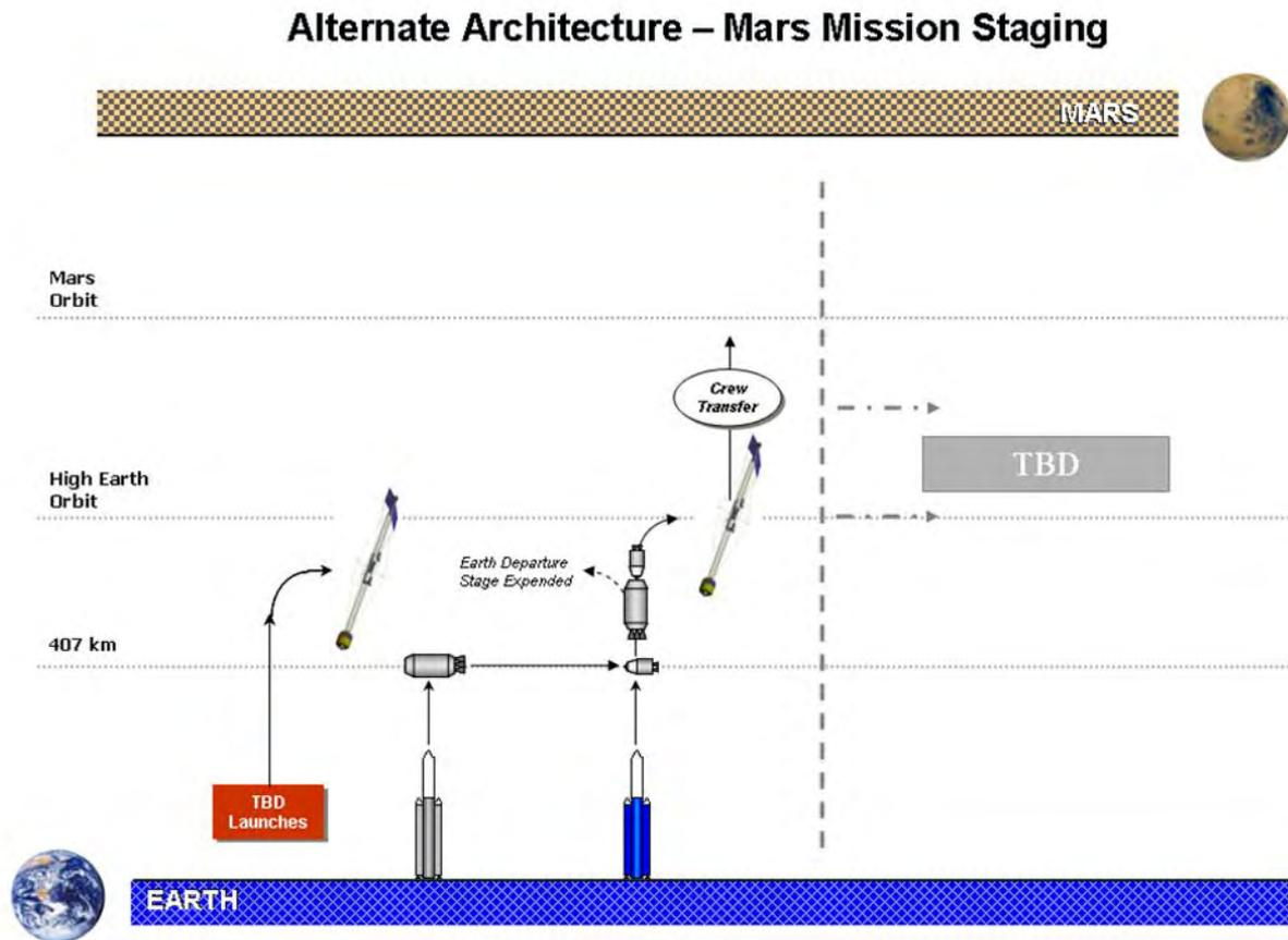
**Figure 11.2.1-1: Mars Mission Staging Architecture Illustration**
