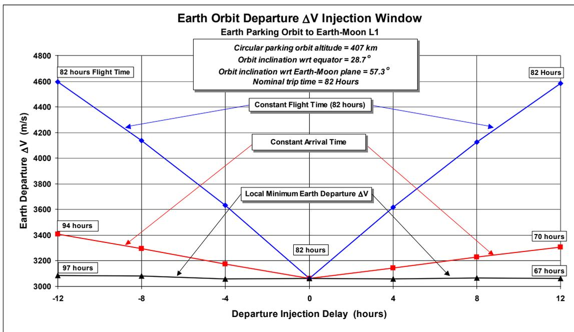
Figure 8.2.1-1b: Earth Departure  $\Delta V$  Cost Versus Earth Departure Time For A Twenty-Four (24) Hour Earth Departure Injection Window
