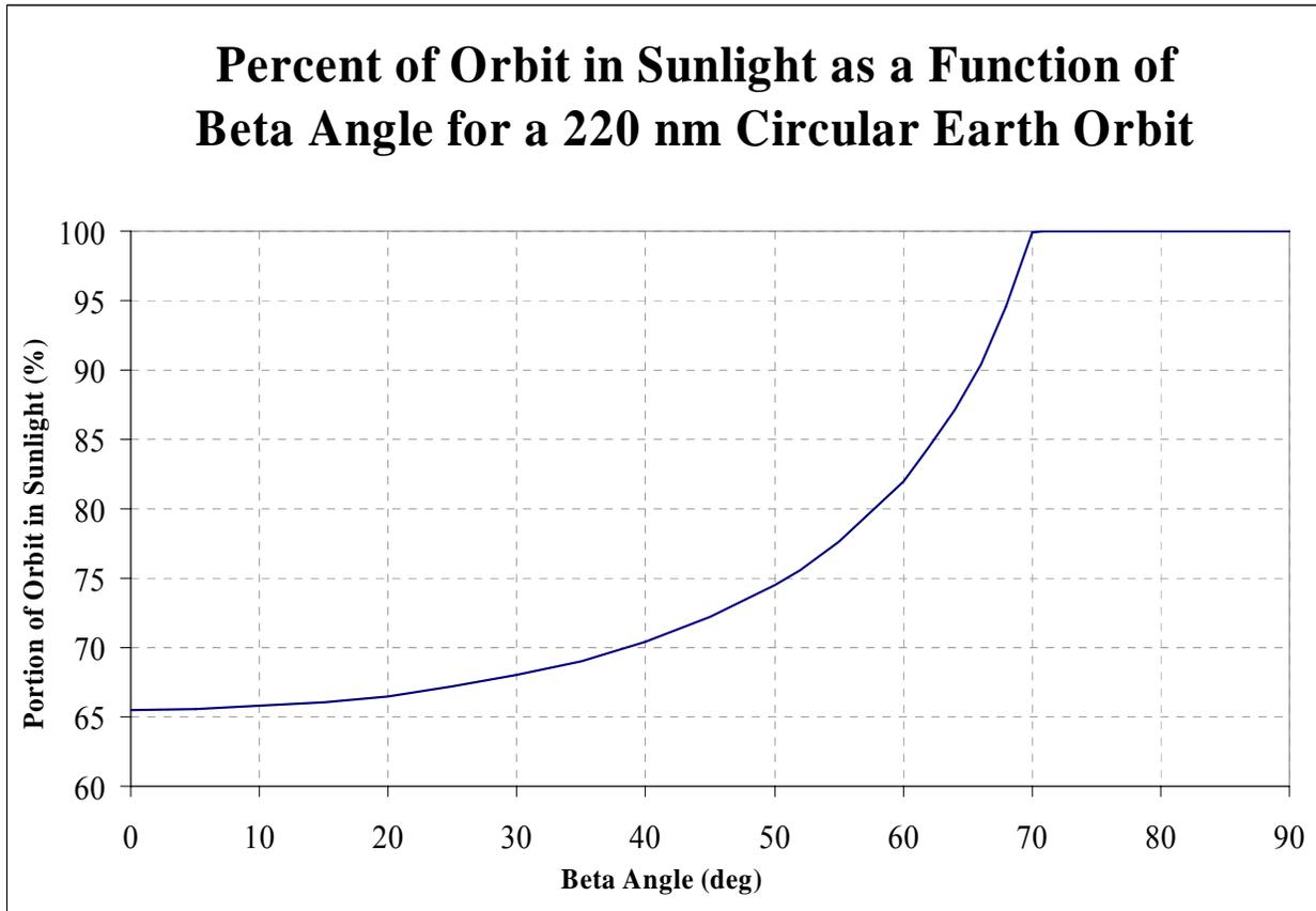
**Figure 20.14.2-1: Portion of Orbit in Sunlight as a Function of Beta Angle**
