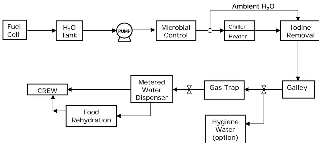
**Figure 20.3.3.2-1: LDRM-2 CEV and Lander Water System Concept**
