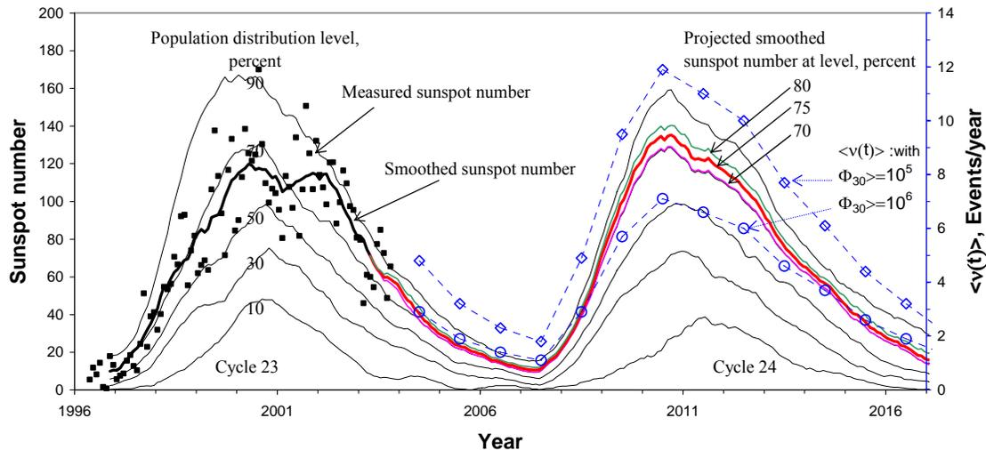
**Figure 20.15.3-3: Sunspot sampling distribution and projections of solar cycles and mean occurrence frequency of SPE**
