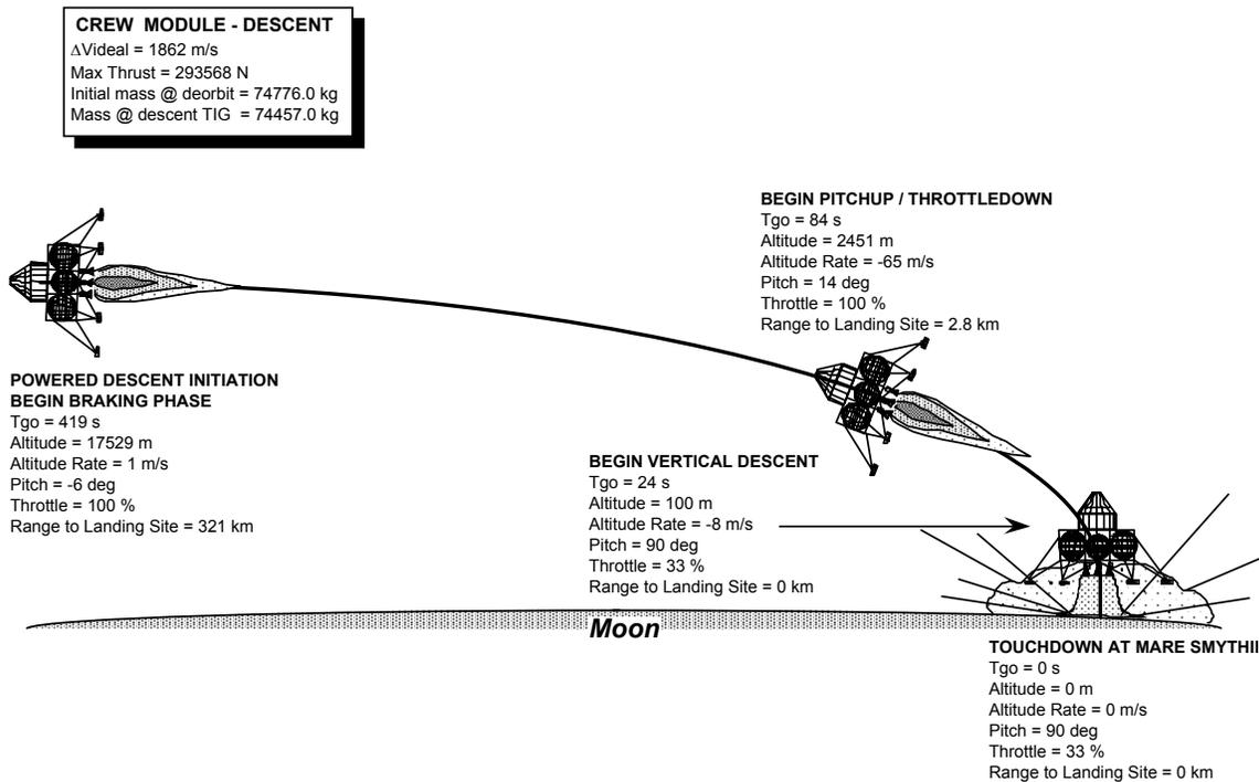
**Figure 8.2.7-2: FLO Powered lunar descent flight profile**
