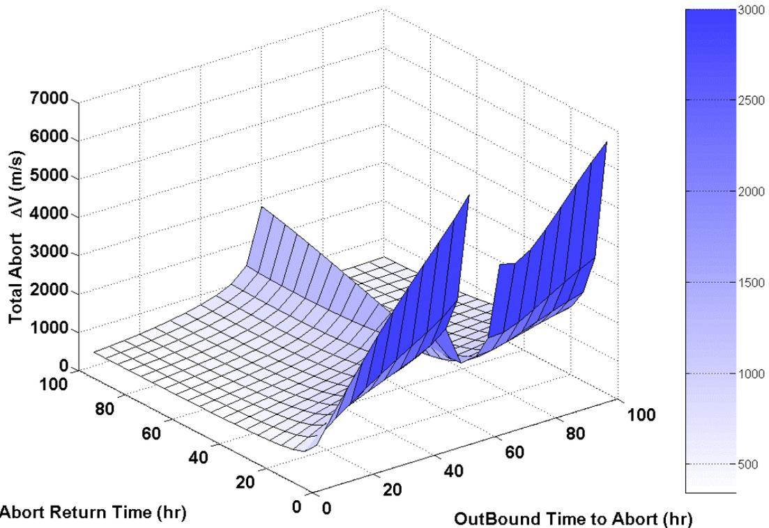
**Figure 8.2.6-3: Mesh Plot of Total Abort  $\Delta V$**
