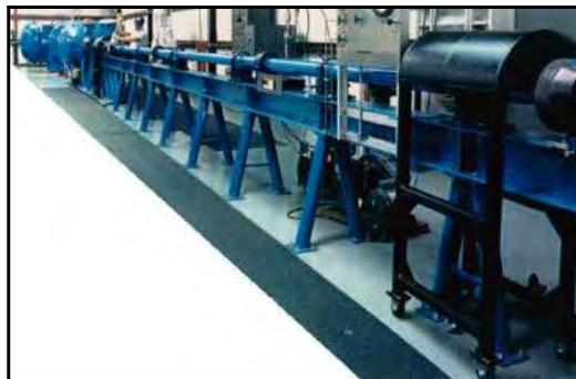
Figure 20.16.2-1: NASA JSC Two Stage Light-Gas Gun
