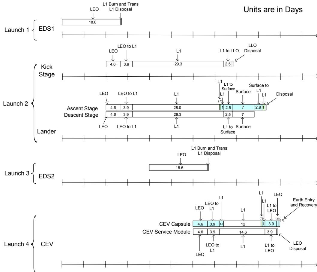
**Figure 16.2-4: Nominal Timeline for the Aerocapture, Phasing, and Land-Landing Architecture**
