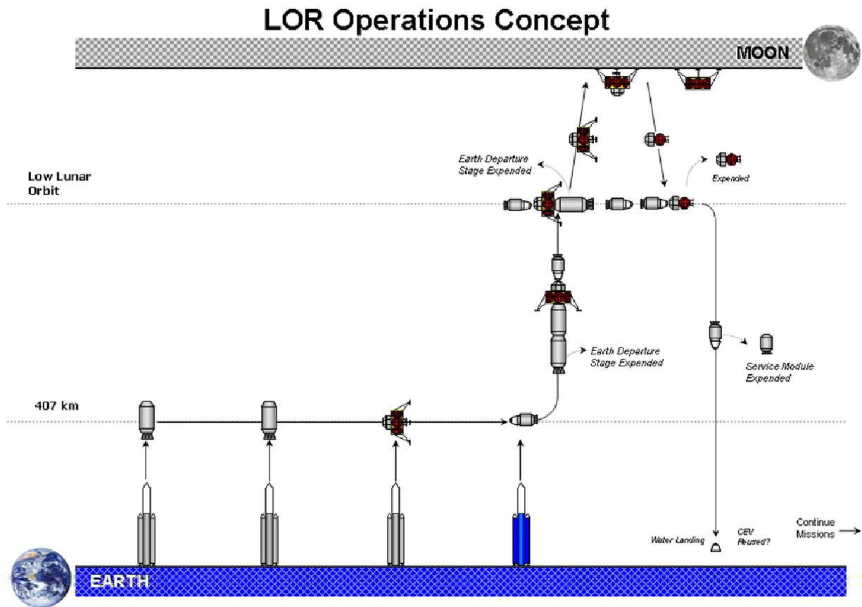
Figure 14.2-2: TRM with Lunar Orbit Rendezvous Architecture Illustration
