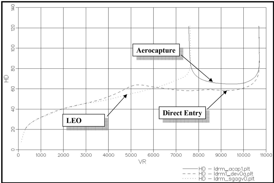
Figure 8.2.10-1: Altitude (km) versus Relative Velocity (m/s)
