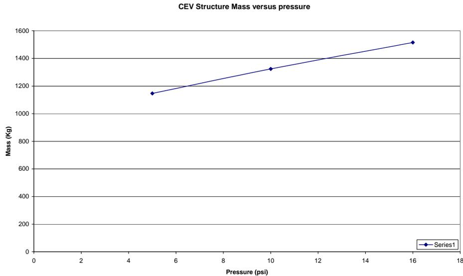
**Figure 19.12.2-2: CEV Cabin Pressure Vessel Mass as a Function of Design Pressure**
