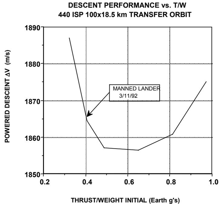
**Figure 8.2.7-1: Powered descent  $\Delta V$  as a function of the initial thrust-to-weight ratio with a legend indicating the vintage of the FLO lander design**
