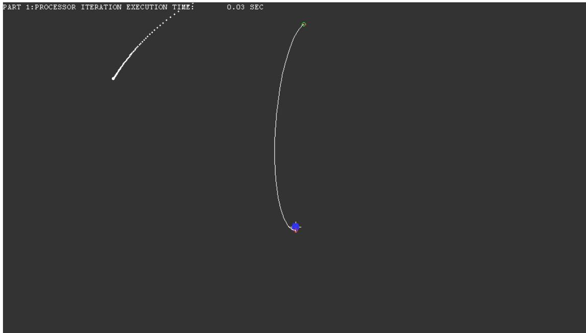
**Figure 8.2.8-2: Stage disposal trajectory to the Earth obtained with Copernicus. Transfer time = 4 days. Disposal maneuver  $\Delta V = 682$  m/s**
