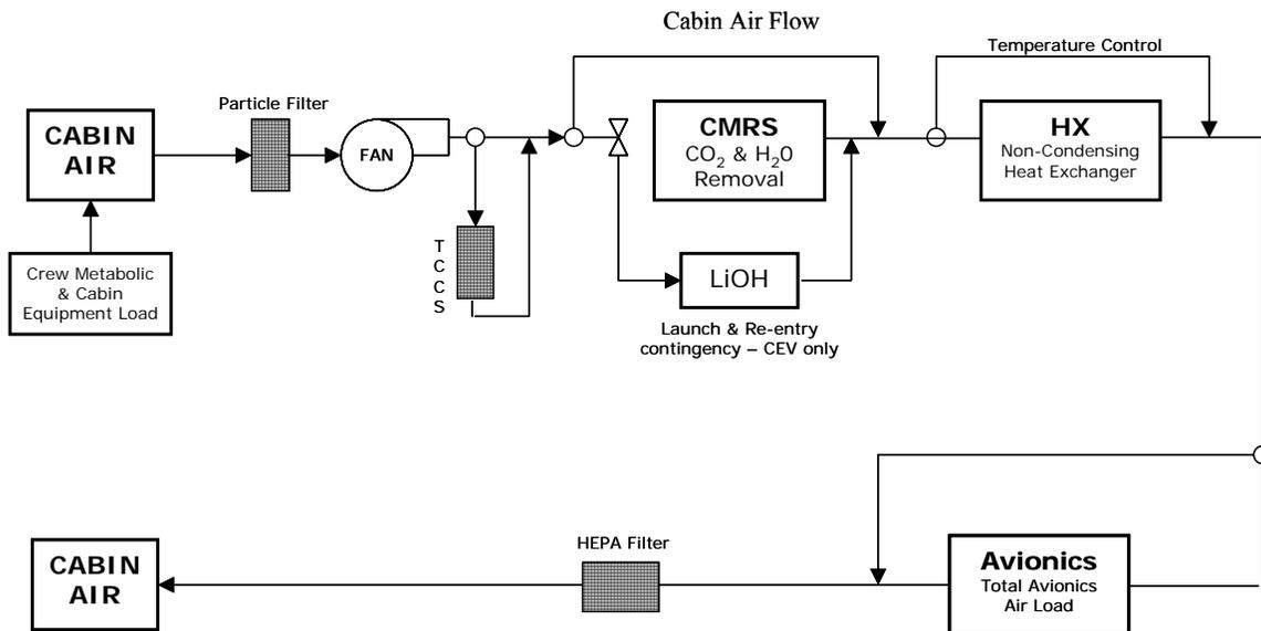
**Figure 20.3.3.1-1: LDRM-2 CEV and Lander Atmosphere Revitalization Concept**
