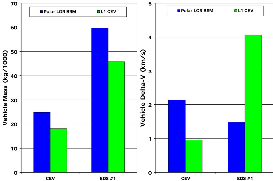
**Figure 9.3-1: CEV/EDS Mass and Delta V Comparison Between the LDRM-2 Phase 2 TRM and L1 CEV Dormant Missions**
