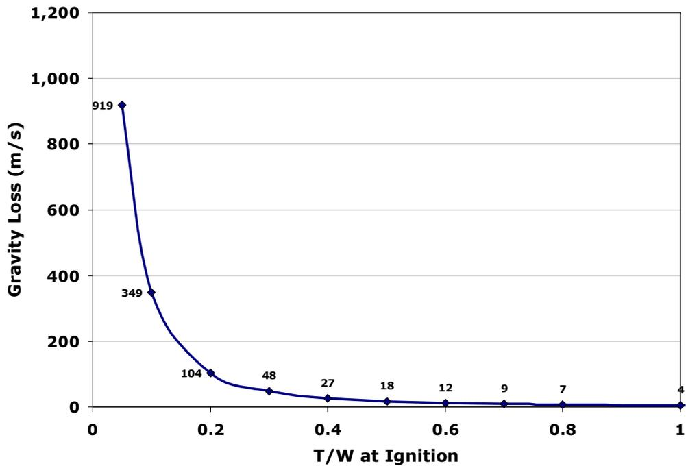
Figure 10.5.4-2: Gravity Loss During Earth Orbit Departure
