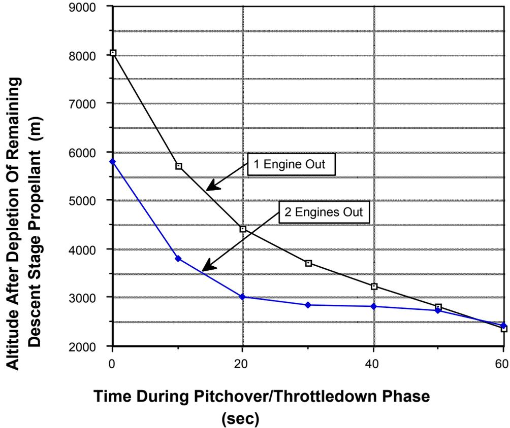
**Figure 8.2.7-11: Altitude after depletion of descent stage propellant versus the time during the 60 second pitchup/throttledown maneuver, for a one and two engine out descent stage assisted ascent to orbit**
