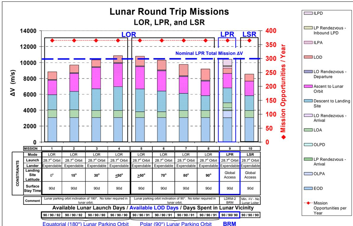
**Figure 6.4-1:  $\Delta V$  cost, constraints, and availability for ten selected round-trip lunar mission scenarios for the Phase 2 study**
