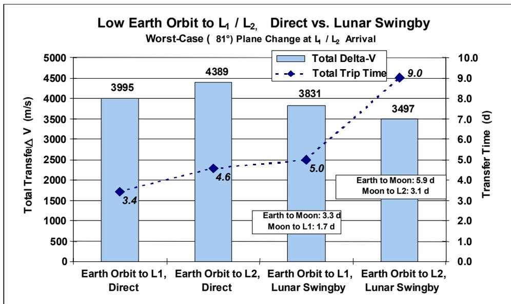
Figure 8.1.2-2:  $\Delta V$  And Trip Time Comparison Of Transfers From Earth Orbit To L1 And L2 Via Either Direct Transfers Or Lunar Swing-By
