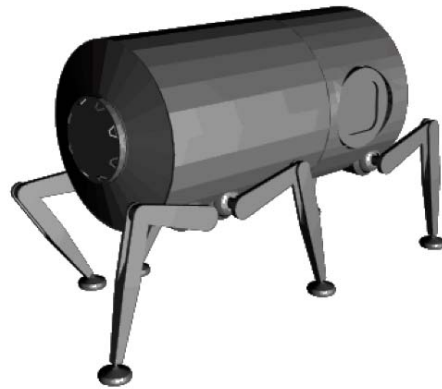
Figure 11: MLH with its articulated legs. (drawing by D. Dunn)
