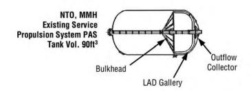
Figure 8-11. Space Shuttle Service Propulsion System Tank Internals
