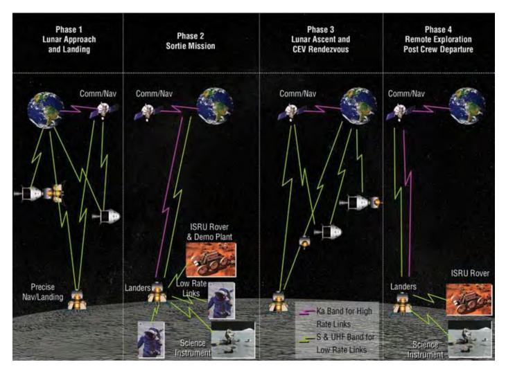
Figure 7-15. Lunar Sortie Surface Communications
