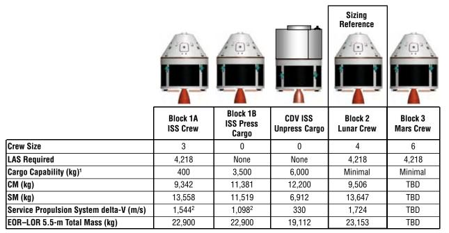
Note 1: Cargo capability is the total cargo capability of the vehicle including Flight Support Equipment (FSE) and support structure. Note 2: A packaging factor of 1.29 was assumed for the pressurized cargo and 2.0 for unpressurized cargo. Extra Block 1A and 1B service propulsion system delta-V used for late ascent abort coverage.
