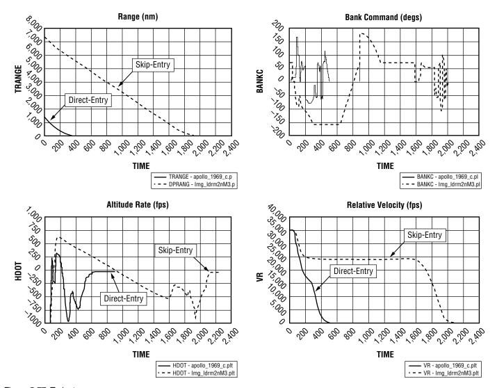
Figure 5-77. Trajectory Comparisons Direct versus Skip-Entry
