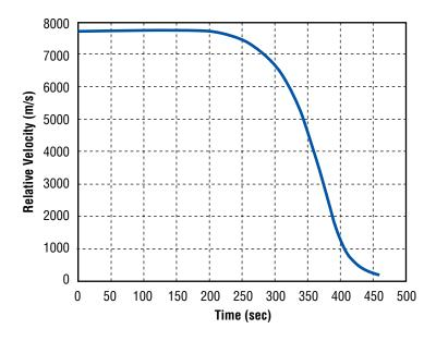
Figure 5-57. Ballistic Entry – Relative Velocity Profile
