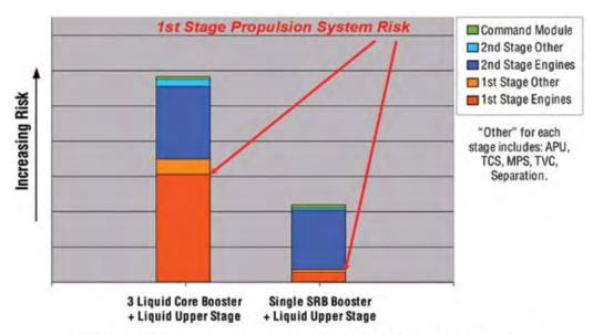
RSRM booster is significantly more reliable than a multi-engine booster
