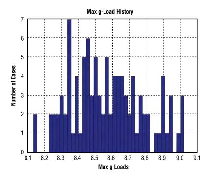
Figure 5-62. Ballistic Entry Monte Carlo G-Load Histogram
