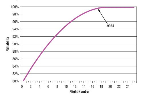
Figure 8-6. Reliability Growth of LOX/Methane Engine
