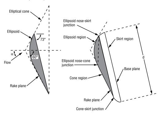
Figure 5-41. AFE-type Shape Parameters
