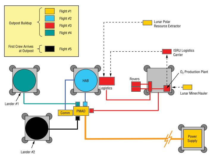
Figure 4-44. Core Outpost Schematic
