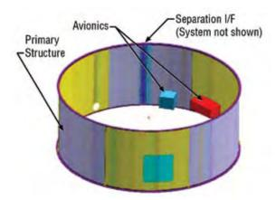
Figure 6-91. SPA Structural Element
