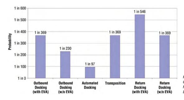
Figure 8-16. Docking Comparisons for Lunar Missions Probability of Docking Failure
