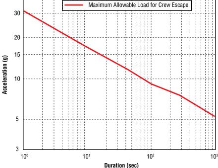
Figure 5-20. Maximum Allowable Load for Crew Escape in the +X Direction (Eyeballs In)
