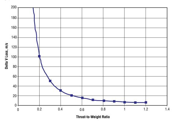
Figure 6-58. Gravity Losses for an EDS Single Burn from 400-km Circular LEO to TLI
