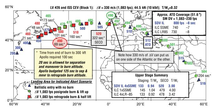
Figure 5-105. Effect of 330 m/s on Landing Areas for LV 26
