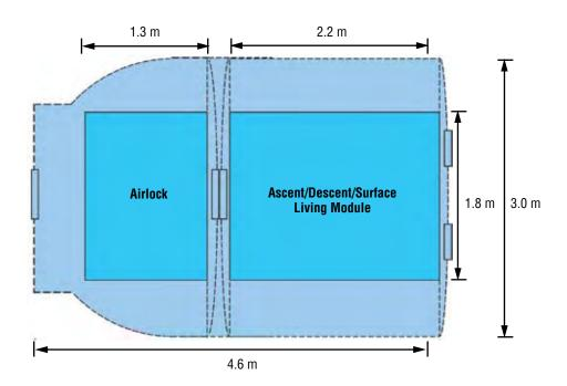
Figure 4-41. LSAM Combined Module Configuration
