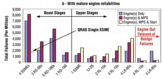
Figure 6-73. Launch Vehicle Stage Reliability Results
