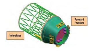
Figure 6-90. Interstage Structural Element Attached to the Forward Frustum
