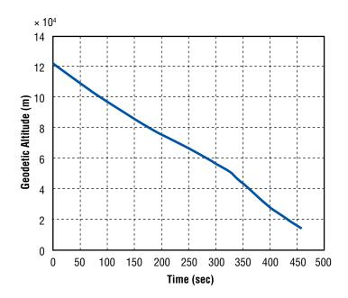
Figure 5-58. Ballistic Entry – Altitude Profile
