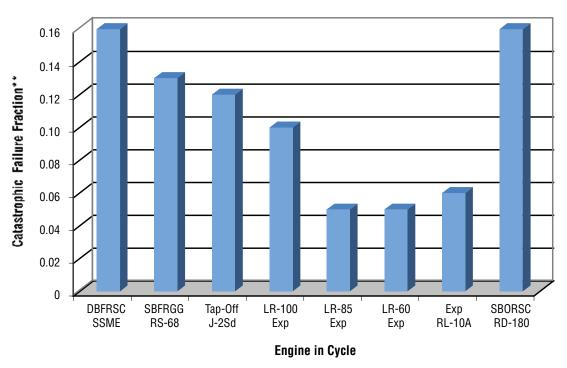
Figure 6-69. Engine Catastrophic Failure Fractions
