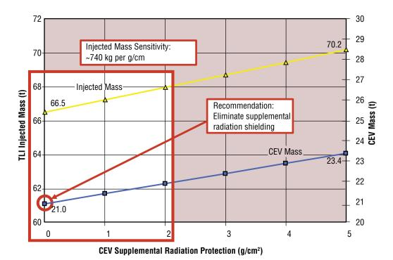
Figure 4-30. 1.5-launch EOR-LOR Sensitivity to CEV Radiation Protection
