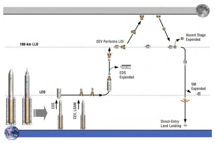
Figure 4-5. EOR-LOR Architecture (Analysis Cycle 1)
