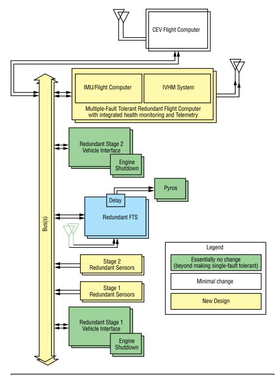
EELV Heritage with dual fault tolerant FC design (single fault-fly mission),
