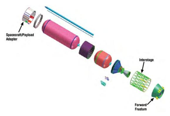
Figure 6-88. Interstages Structural Elements Within the Upper Stage
