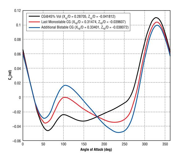
Figure 5-31. Pitching Moment Coefficient Curves for the Baseline Capsule
