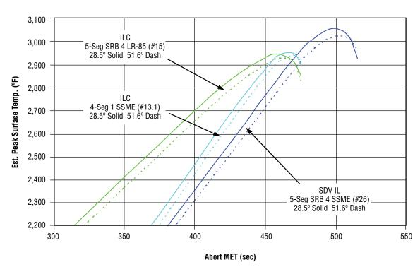
Figure 5-97. Maximum Surface Temperatures for Ballistic Aborts from Shuttle-Derived Boosters
