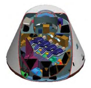
Figure 4-23. EOR-Direct Return CEV CAD Cutaway Showing Four-Crew Earth Launch Configuration
