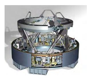
Figure 5-47. LIDS Docking/Berthing Mechanism
