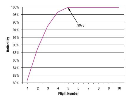
Figure 8-7. Reliability Growth of SSME Air Start (Pump-fed LOX/ Hydrogen)
