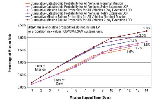
Figure 4-35. Delta P(LOC) and P(LOM) for Extending Orbital Loiter Prior to Lunar Descent
