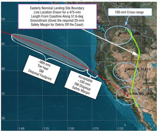
Figure 5-49. Maximum Landing Site Boundary for a 0.4 L/D CM Returning from a 51.6deg Space Station Orbit
