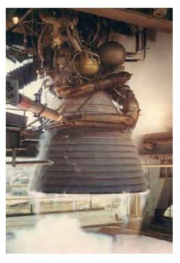
Figure 8-14. J–2S Test Firing
