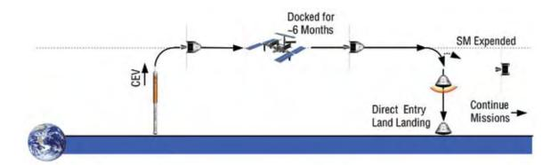
checks, and undocks from the station. The CEV departs the vicinity of the ISS and conducts an onboard-targeted (ground-validated) deorbit burn. After burn completion, the CEV SM is discarded, and the return component is maneuvered to the proper entry interface attitude for a guided entry to the landing site. The CEV performs a nominal landing at the primary land-based landing site.
