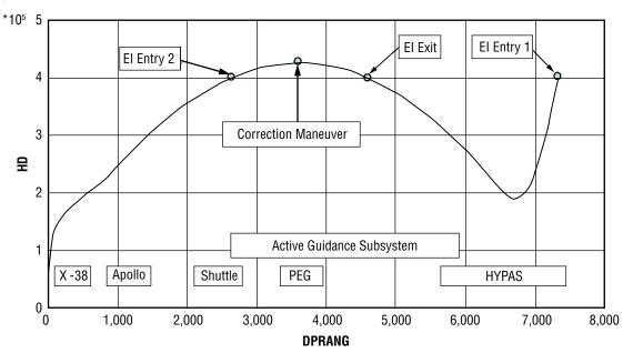
Figure 5-67. SPASE Nominal Flight Geodetic Altitude (ft) versus Range (nmi) to Landing Site
