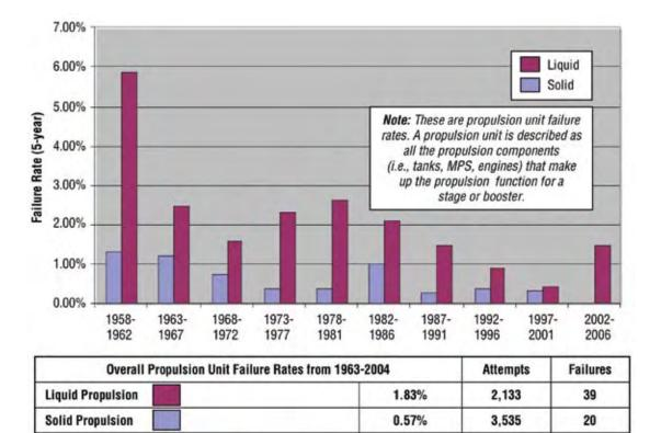
Figure 6-76. Failure Rates of Solid and Liquid Propulsion Systems
