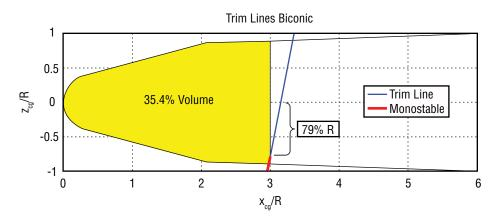
Figure 5-16. Biconic Shape with Trim Line
