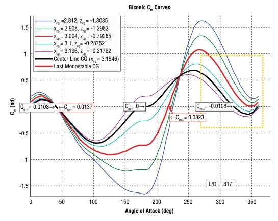
Figure 5-17. C<sub>m</sub> Curves for Biconic Vehicle
