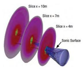
Figure 8-9. Contours of Constant Axial Velocity
