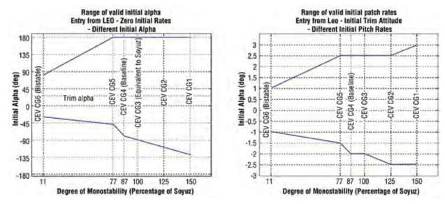
Figure 5-36. Valid Initial Attitudes and Pitch Rates in Entry from LEO versus Different Degrees of Monostability
