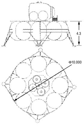
Figure 4-38. LV Shroud Diameter Influence on LSAM Tank Configuration
