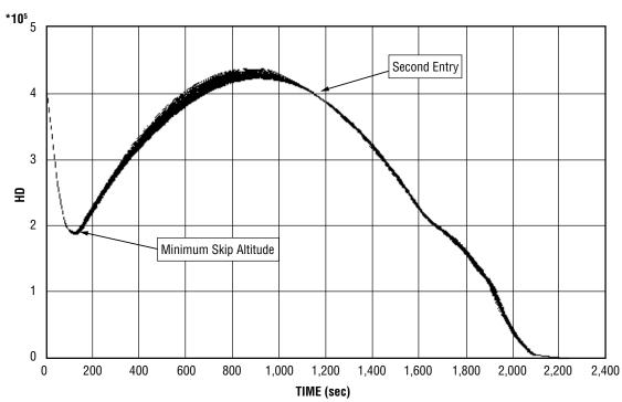
Figure 5-74. Geodetic Altitude (ft) versus Time (sec)—Dispersed Flight (100 Cases)
