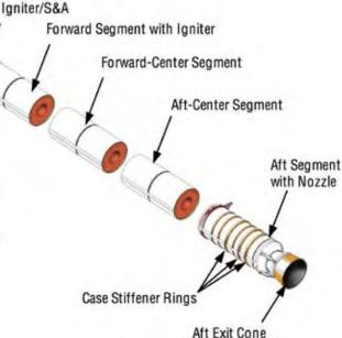
Figure 6-75. Basic Elements of a Shuttle RSRB
