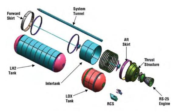
Figure 6-87. Upper Stage Structural Elements
