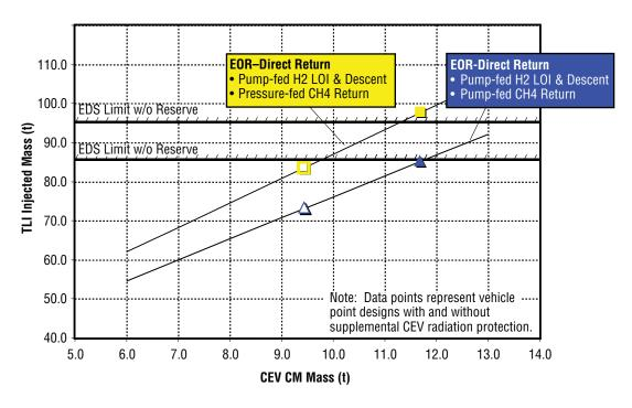
Figure 4-10. TLI Injected Mass versus Crew Compartment Mass, With and Without 5.0 g/cm² Supplemental Radiation Protection
