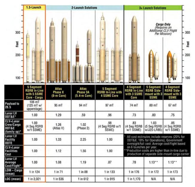
Figure 1-28. Lunar Cargo Launch Comparison
