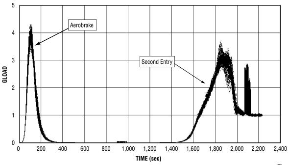
Figure 5-71. SPASE Dispersed Flight Acceleration (g's) versus Time (sec) (100 Cases)
