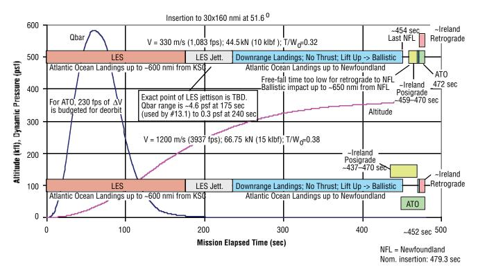
Figure 5-106. Abort Modes for Launch Vehicle 13.1 with the ISS CEV and Two Propulsion System Configurations
