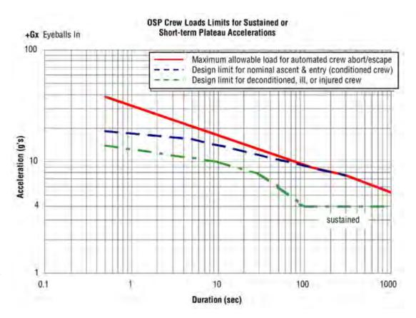
Figure 5-15. Example of NASA Standard 3000 Crew Load Limits
