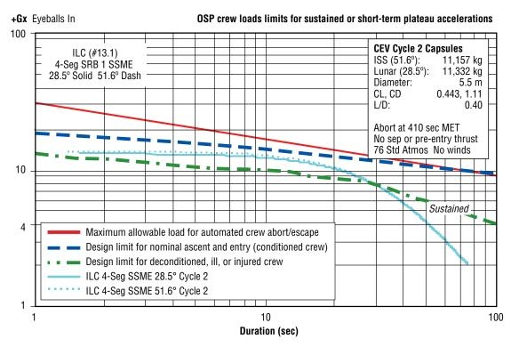
Figure 5-102. Worst Case Ballistic Load Durations for Cycle 2 CEV and LV 13.1
