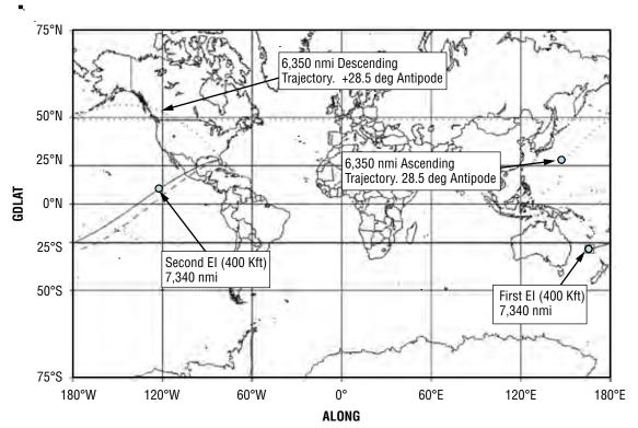
Figure 5-66. SPASE Nominal Flight Groundtrack to KSC
