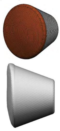
Figure 5-32. Baseline Axisymmetric Shape CBAERO Grid
