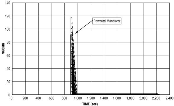
Figure 5-72. SPASE Powered Maneuver Delta Velocity Required (fps) versus Time (sec) (100 Cases)
