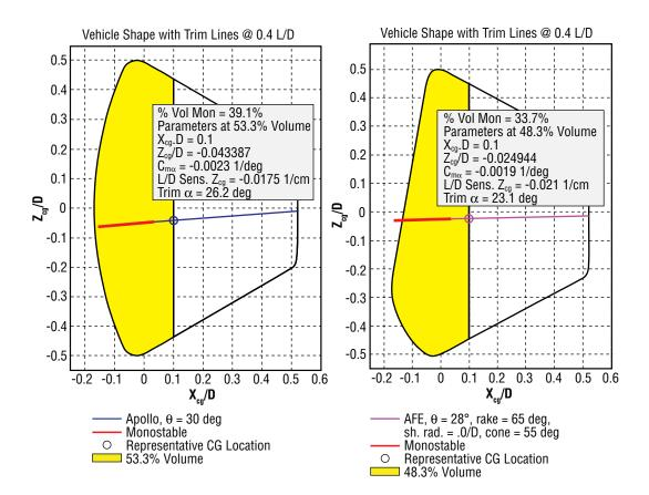
Figure 5-42. Alternate Symmetric and AFE Heat Shield Vehicles
