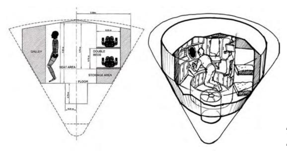
Figure 4-17. Split-Volume EOR-Direct Return CEV Layout
