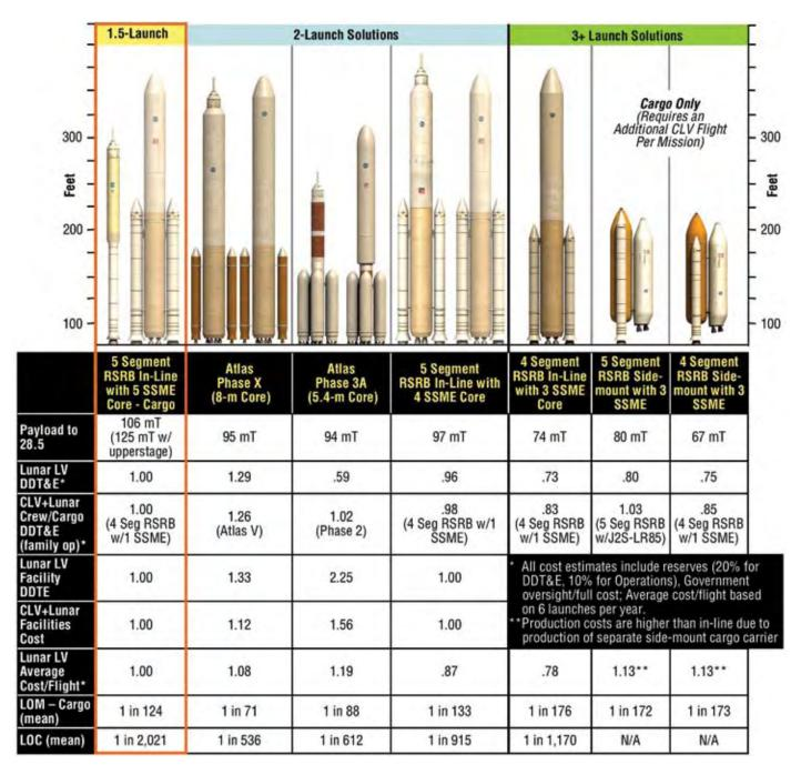
Figure 6-96. Lunar Cargo Launch Comparison
