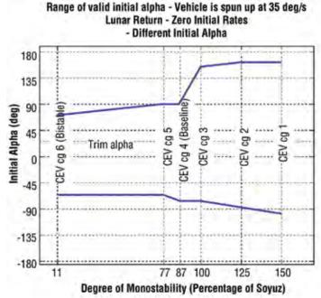
Figure 5-40. Valid Initial Attitudes and Pitch Rates Entry from Lunar Return with Spin Up (35 deg/s) versus Different Degrees of Monostability
