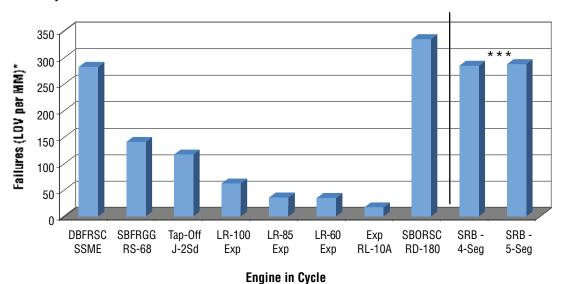
Figure 6-68. Engine Catastrophic MTBFs
