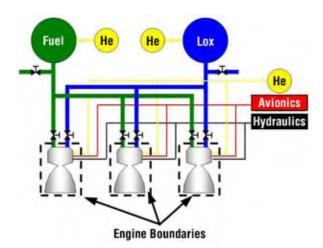
Figure 8-22. Liquid Propulsion System Schematic
