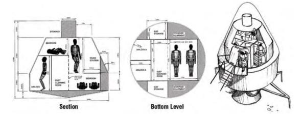
Figure 4-21. Single-Volume CEV Study Design Layouts
