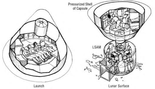
Figure 4-20. Split-Volume EOR-Direct Return CEV + Airlock Module Layout by Flight Phases
