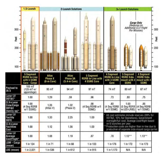
Figure 6-18. Lunar Cargo Launch Comparison
