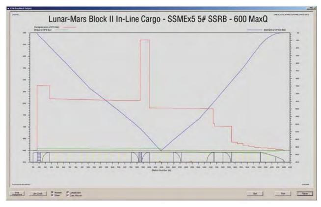
Figure 6-40. CaLV Structural Loads Analysis Results
