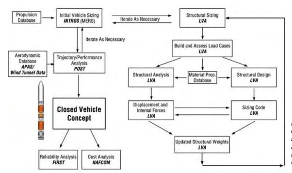
Figure 6-1. Vehicle Conceptual Sizing and Performance Analysis Flow for Earth-to-Orbit (ETO) LVs
