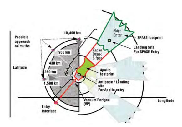
Figure 5-87. Entry Footprint with Co-azimuth Control (Direct-Entry and Skip-Entry), 0.4 L/D
