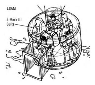
Figure 4-18. Split-Volume EOR-Direct Return CEV Airlock Module
