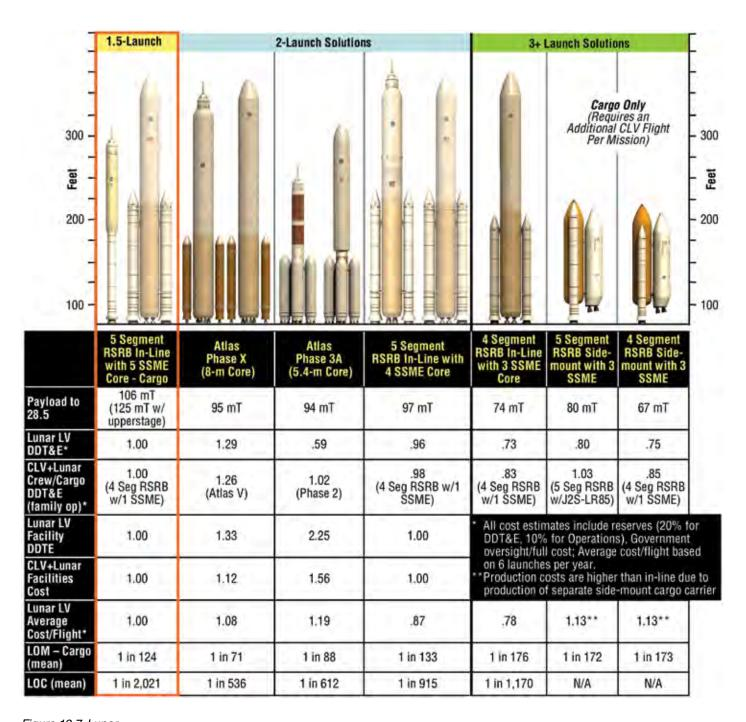
Figure 12-7. Lunar Cargo Launch Systems Comparison
