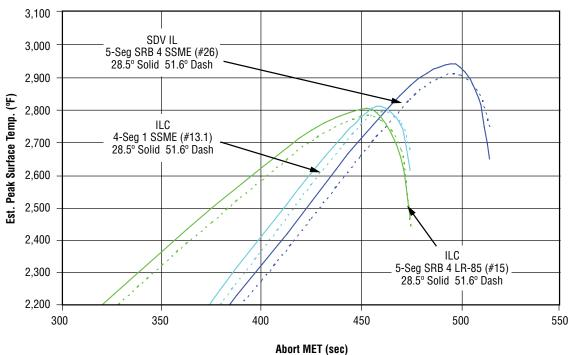
Figure 5-98. Maximum Surface Temperatures for Lift-up Aborts from Shuttle Derived Vehicles
