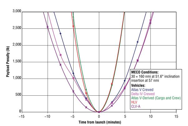
Figure 6-6. Launch Window Payload Penalties (ISS Mission)
