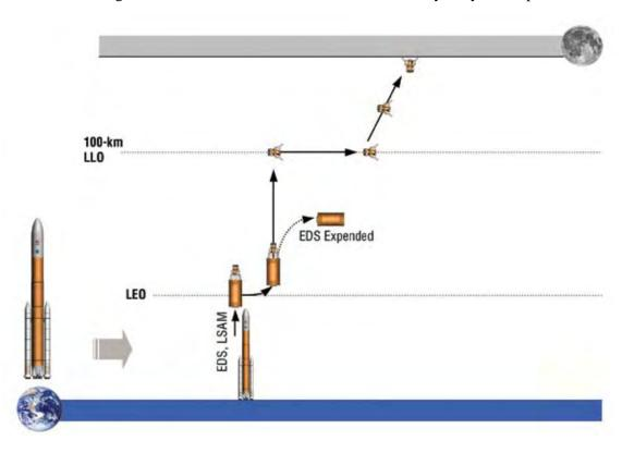
Figure 1-6. Lunar Outpost Cargo Delivery DRM
