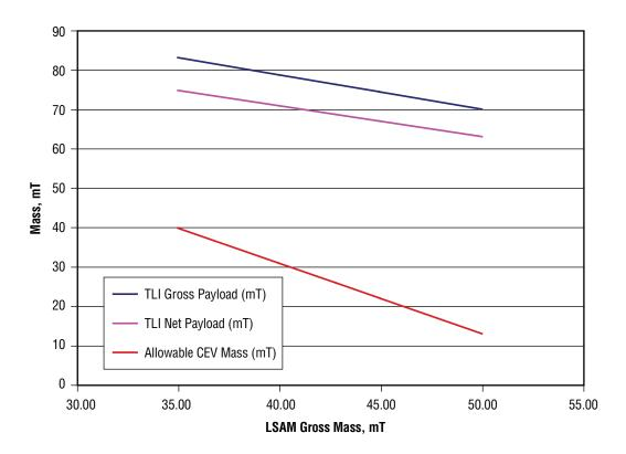
Figure 6-38. 1.5-Launch Solution Allowable Masses as a Function of LSAM Mass
