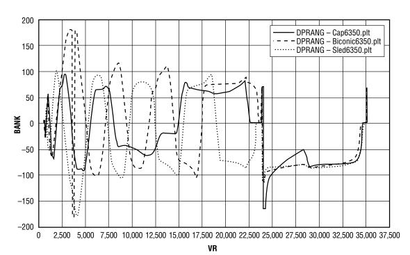
Figure 5-82. Bank Angle versus Relative Velocity (fps)
