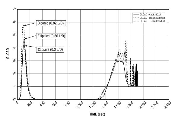
Figure 5-79. Total Aerodynamic Acceleration (g's) versus Time from El (sec)
