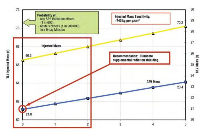
Figure 8.3. 1.5-Launch Solution Sensitivity to CEV Radiation Shielding
