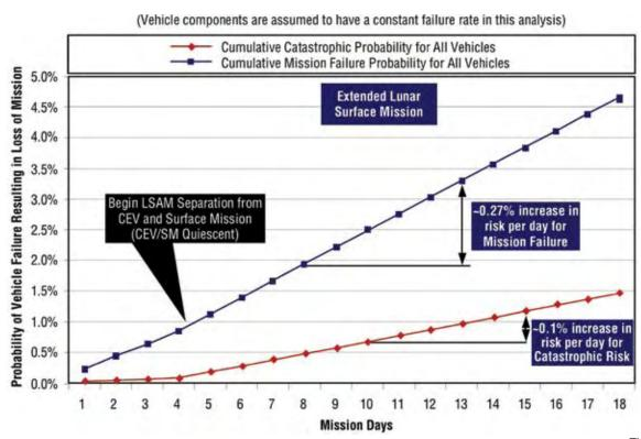
Figure 8-31. Mission Failure Probabilities Over an Extended Mission
