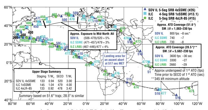
Landing areas are indicated for ballistic abort entries with no separation or post-abort thrust
