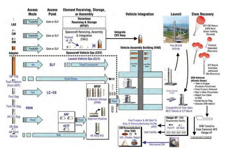
Figure 7-1. Defining the CEV/CLV Operations Concept
