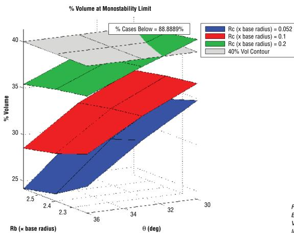
Figure 5-27. Example of Effect of Parameterized Variables on Quantity of Interest (Monostability)
