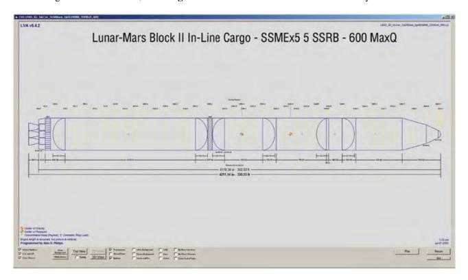
Considerable effort was used to optimize this particular vehicle for payload to TLI. A max q of 600 lb/ft² was used (as calculated by the Program to Optimize Simulated Trajectories (POST) tool) instead of the 750 normally used for this class of vehicle. Also, a more efficient conical thrust structure was used for the EDS instead of the standard cruciform. The core was also re analyzed for the loads in this particular case.
