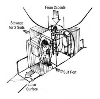
Figure 4-19. Alternative Airlock Module Layout
