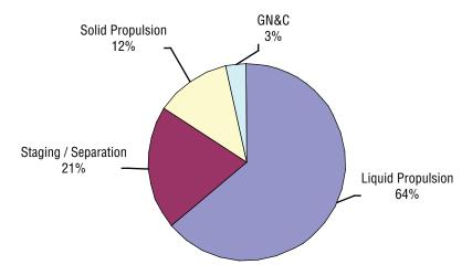
Notes: Percentages are based on the mean LOM failure probability. SSME burntime is 336 seconds.
