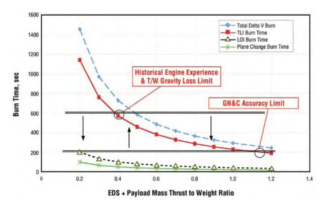
Figure 6-59. Bounding Limits on EDS Thrust and Engine Thrust
