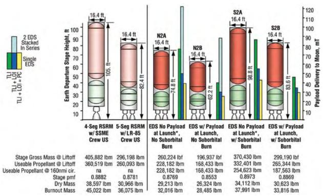
Figure 6-54. EDS Sizes Launched on In-Line SDV with 5-Segment RSRB
