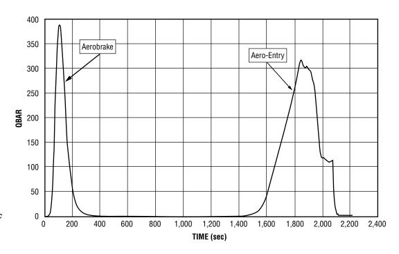
Figure 5-69. SPASE Nominal Flight Dynamic Pressure (psf) versus Time (sec)
