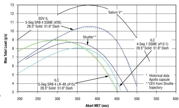
Figure 5-96. Lift-up Loads for Aborts from SDVs
