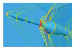
Figure 8-10. Aerodynamic Loads on Steady-State Ascent
