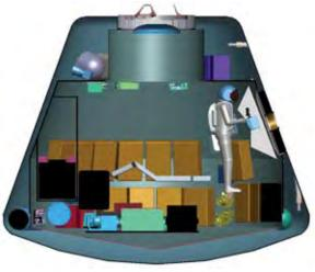
Figure 4-24. EOR-Direct Return CEV CAD Section Showing Lunar Ascent and Descent Pilot Position
