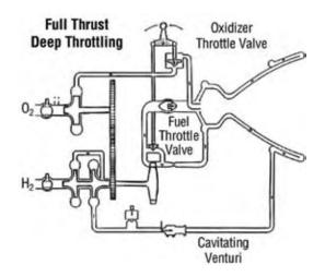
Figure 8-12. RL–10 Throttling Approach
