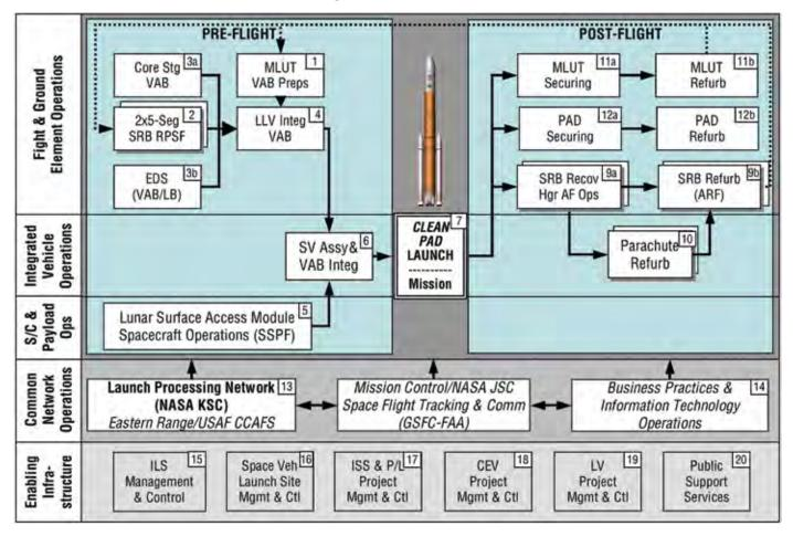
Figure 7-6. LSAM/CaLV Ground Operations Architecture
