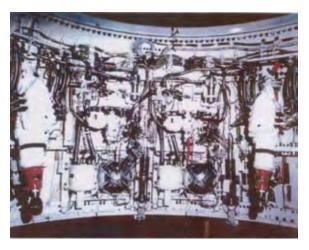
Figure 7-10. SRB Aft Skirt Thrust Vector Control Installation
