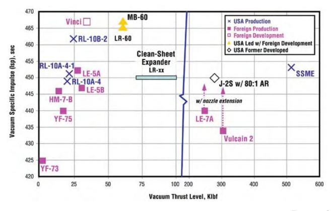
Figure 6-57. Candidate LOX/LH2 Engines for an Upper Stage and Earth Departure Stage Main Engine
