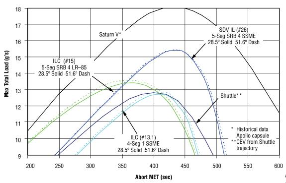
Figure 5-95. Ballistic Loads for Aborts from Shuttle-Derived Boosters
