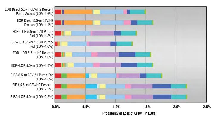
Figure 4-29. Analysis Cycle 2: LOC Comparison
