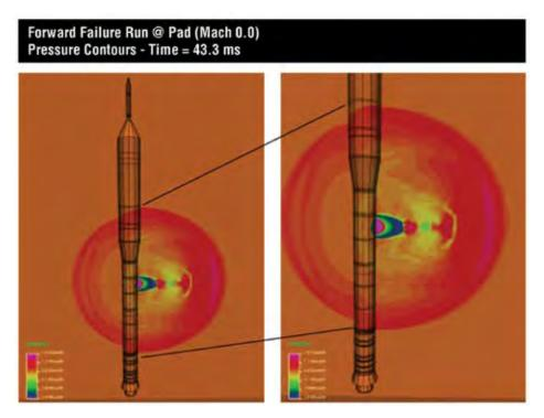
Figure 6-81. Worst-Case Condition of a Forward Segment Rupture on the Pad
