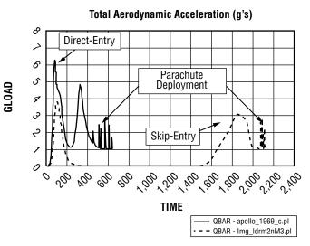
Figure 5-76. Trajectory Comparisons Direct versus Skip-Entry
