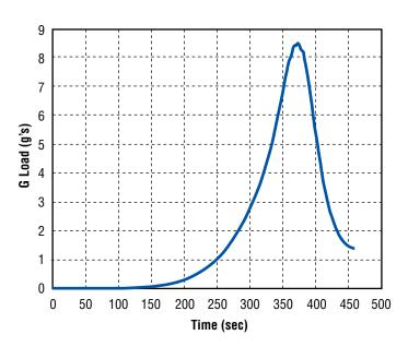
Figure 5-59. Ballistic Entry – g-Load Profile
