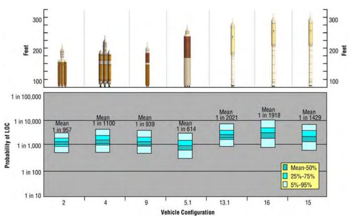
Figure 8-18. CLV LEO Launch Systems LOC
