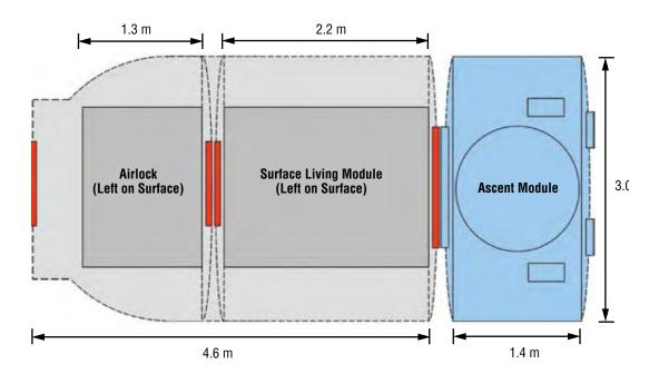
Figure 4-39. LSAM Minimized CM Vehicle Configuration
