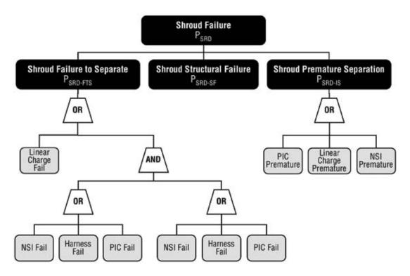
Figure 6-74. Payload Shroud Fault Tree
