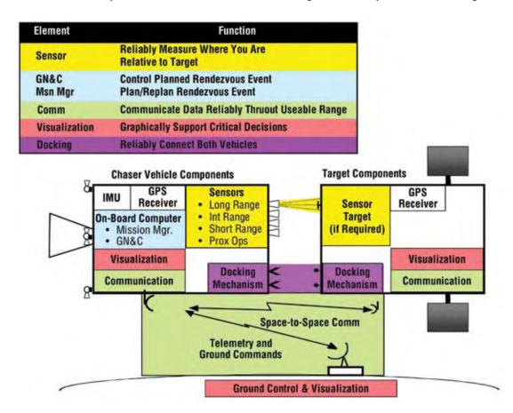
Figure 6-22. An AR&D System's Chaser and Target Components
