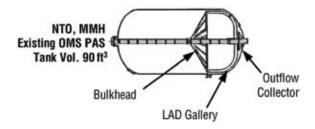
Figure 4-14. OMS Tank Internals Showing LAD Approach
