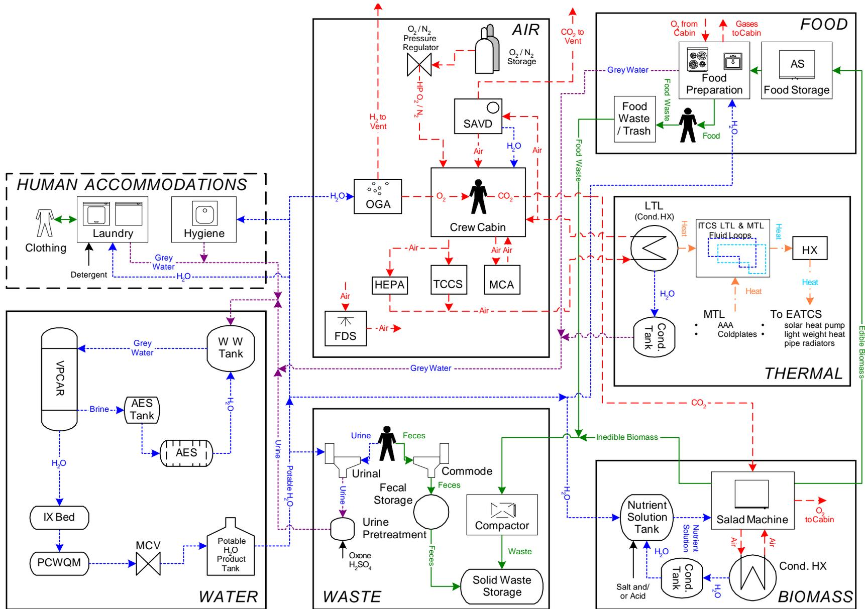
Figure 3.4 Life Support Concept for the Mars Transit Vehicle in the Mars Dual Lander Architecture Using ALS Technologies (without ISRU)
