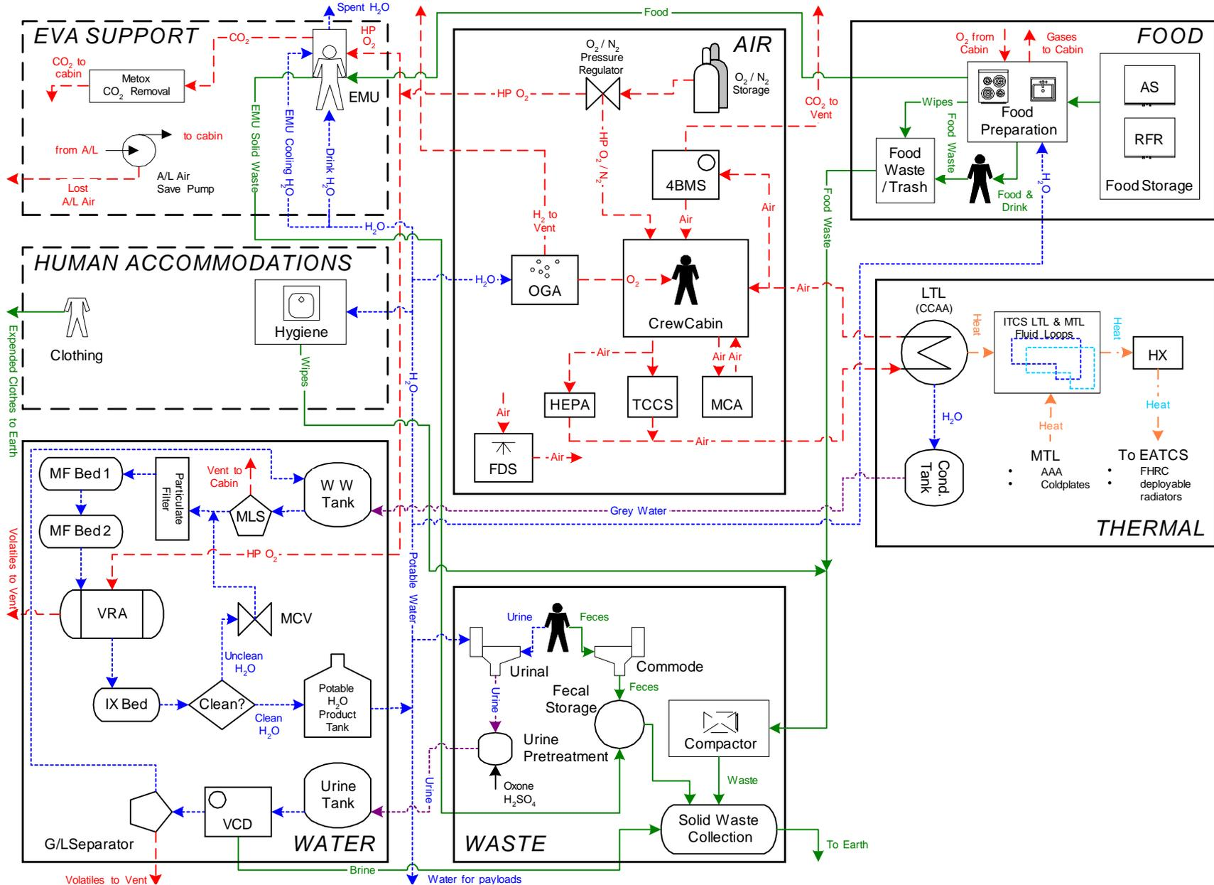
Figure 2.4 Life Support Design for Phase 3 of the US Segment of the International Space Station Mission Using ISS Baseline Technologies.
