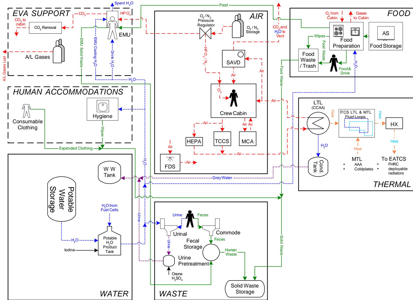
Figure 3.3 Life Support Design for the Mars Descent/Ascent Lander in the Mars Dual Lander Architecture Using ISS Technologies (without ISRU)
