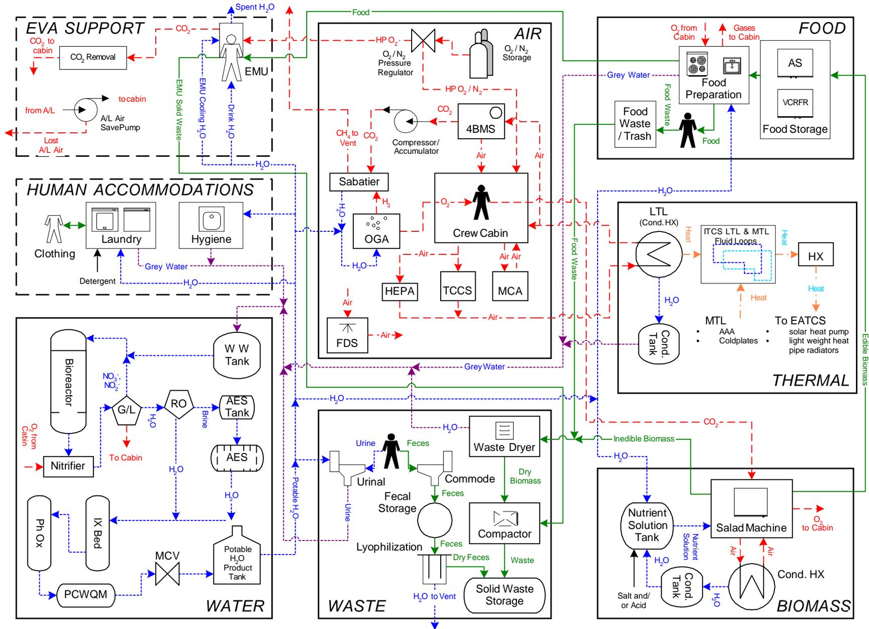
Figure 3.5 Life Support Concept for the Surface Habitat Lander in the Mars Dual Lander Architecture Using ALS Technologies (without ISRU)
