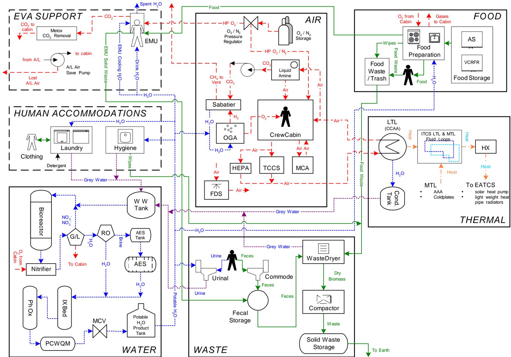
Figure 2.6 Life Support Concept for Post Phase 3 of the United States On-orbit Segment of the International Space Station Using ALS Technologies.
