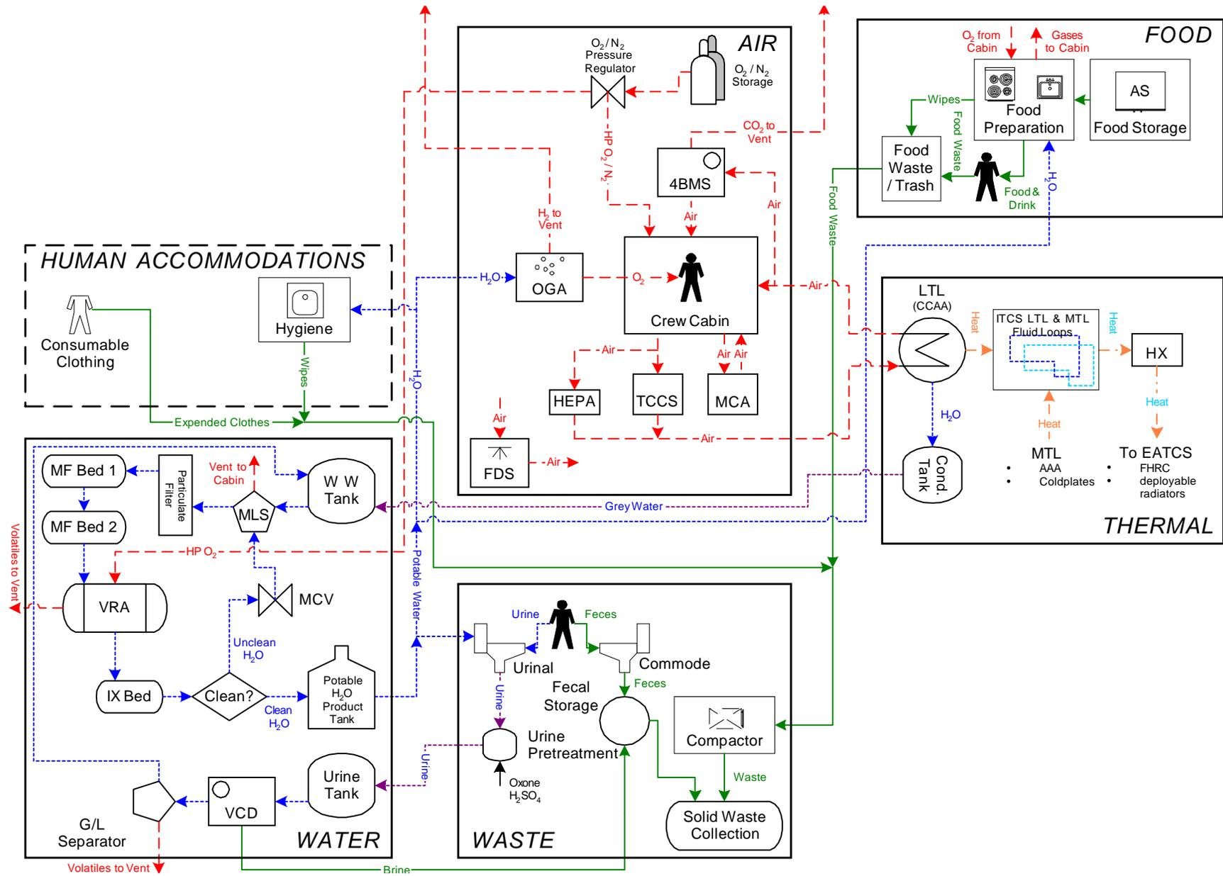
Figure 3.1 Life Support Design for the Mars Transit Vehicle in the Mars Dual Lander Architecture Using ISS Baseline Technologies.
