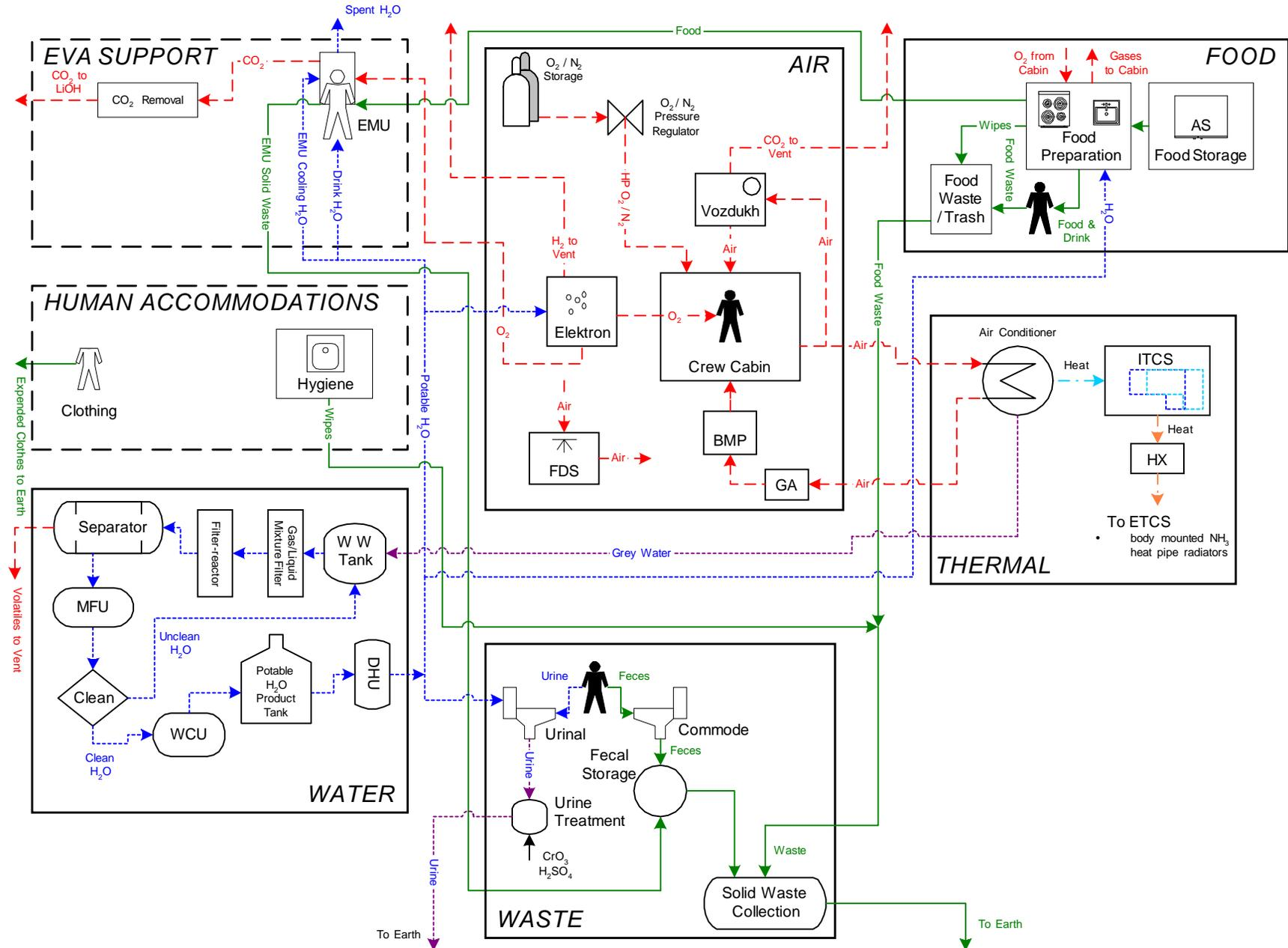
Figure 2.1 Life Support Design for Phase 2 of the Russian Segment of the International Space Station Mission Using ISS Baseline Technologies.
