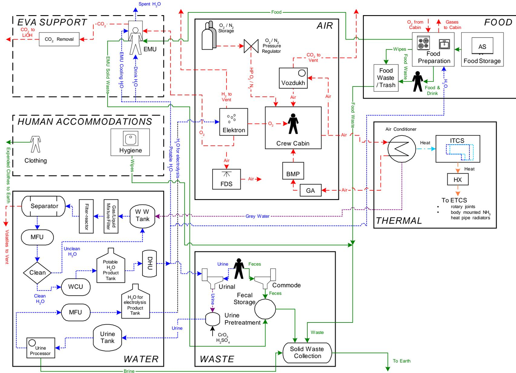
Figure 2.2 Life Support Design for Phase 3 of the Russian Segment of the International Space Station Mission Using ISS Baseline Technologies.
