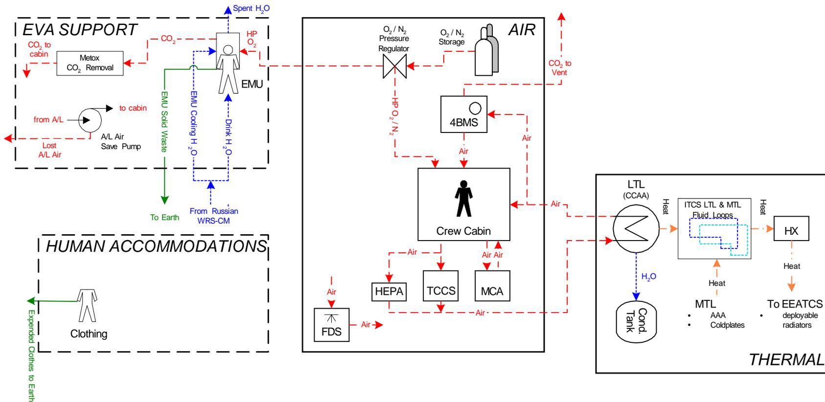
Figure 2.3 Life Support Design for Phase 2 of the US Segment of the International Space Station Mission Using ISS Baseline Technologies.
