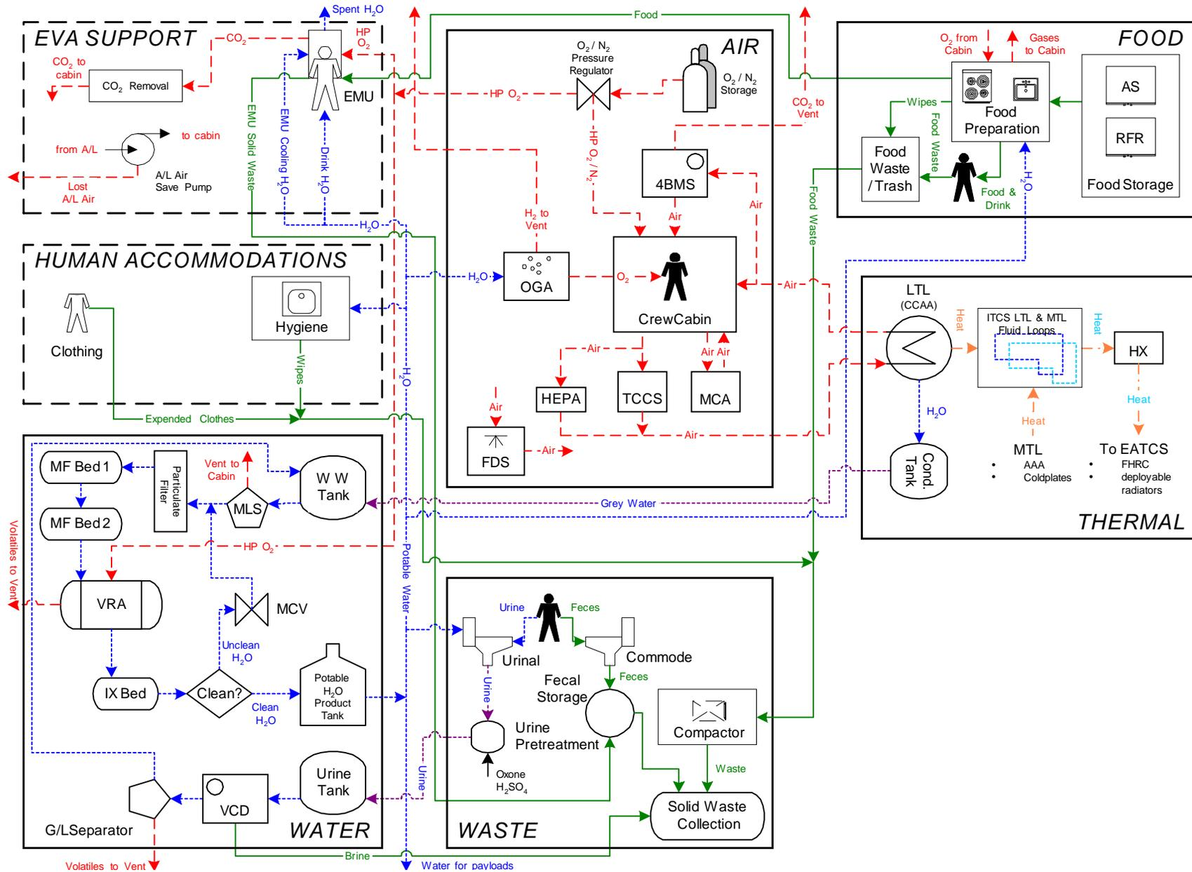
Figure 3.2 Life Support Design for the **Surface Habitat Lander** in the Mars Dual Lander Architecture Using **ISS Baseline Technologies**.
