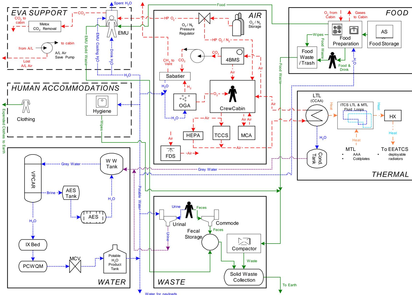
Figure 2.5 Life Support Concept for Post Phase 2 of the United States On-orbit Segment of the International Space Station Using ALS Technologies.
